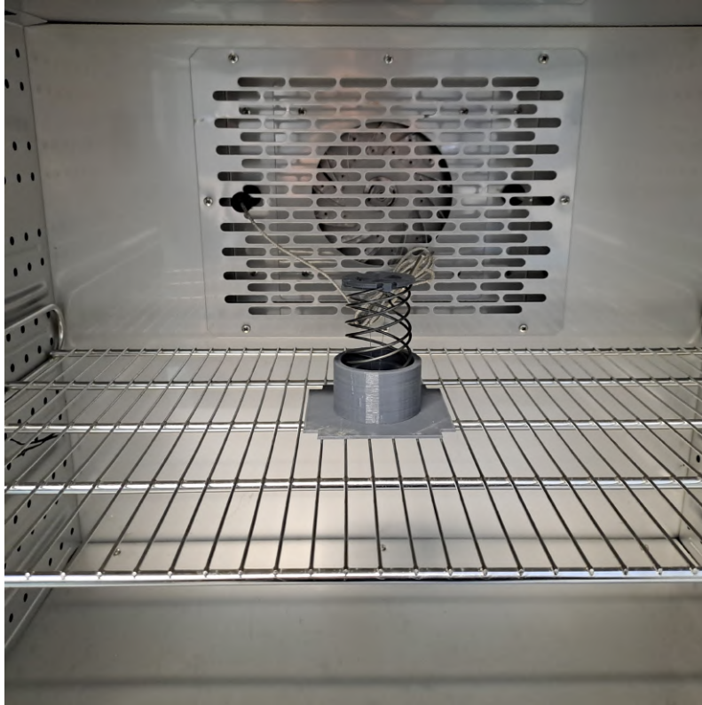
Figure 6.19: Antenna System Post Thermal Test
