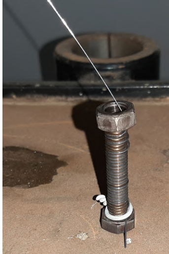
Figure 3.10: Trained Specimen Left to Air Cool
