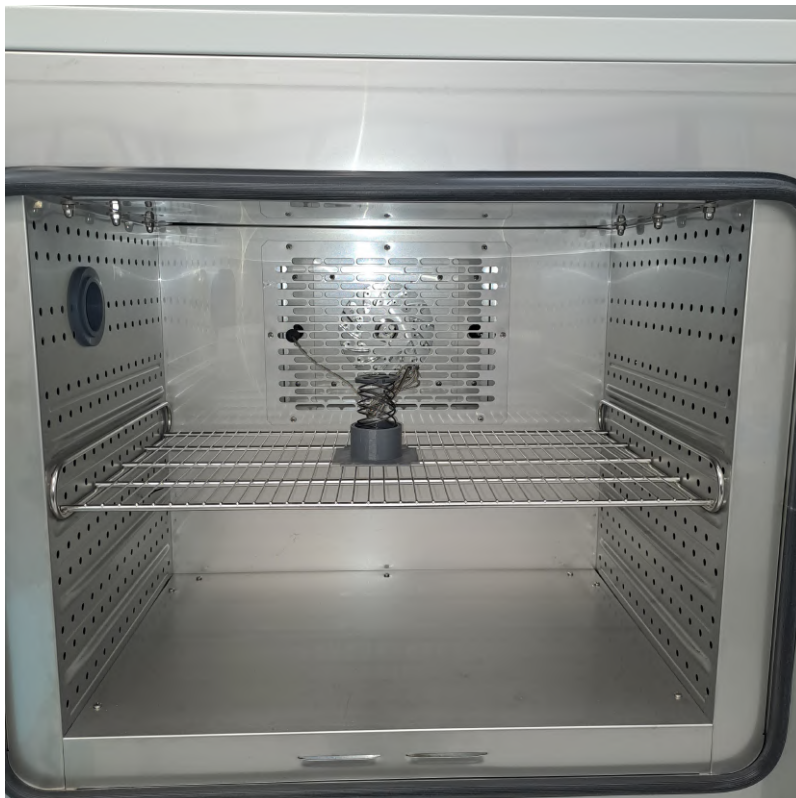
Figure 6.16: QHA Placed in Thermal Chamber
