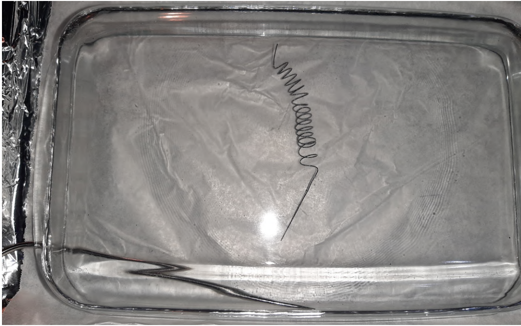
Figure 3.14: Remembered Shape at Austenite Finish Temperature
