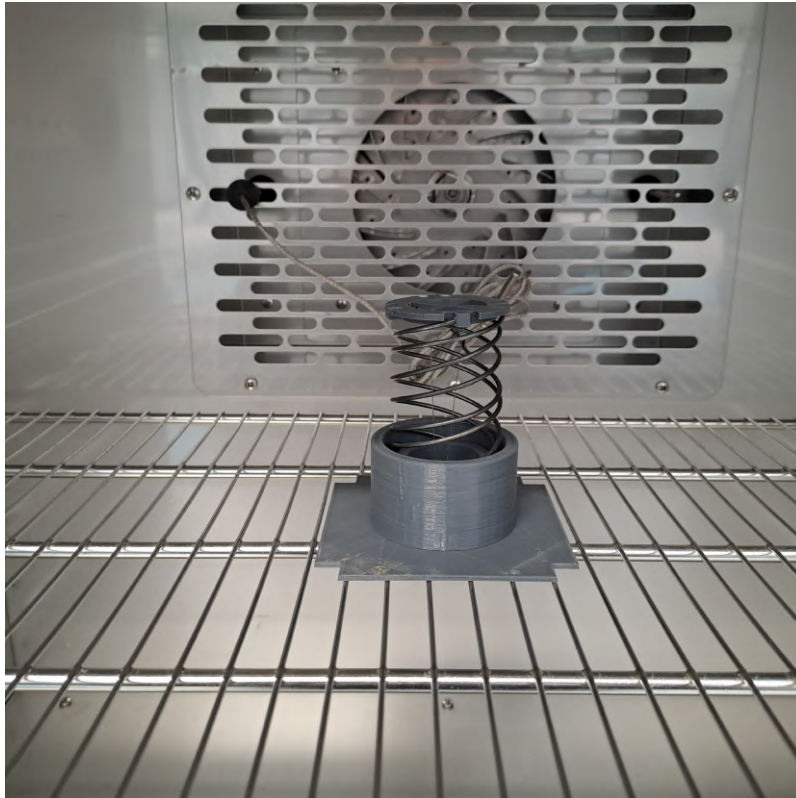
Figure 6.17: QHA Placed in Thermal Chamber Close Up
