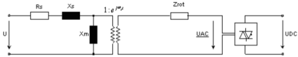
Figure 3.8: Doubly-Fed Induction Machine circuit
