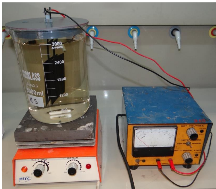
Photo 3.6: Electrochemical oxidation batch reaction.
