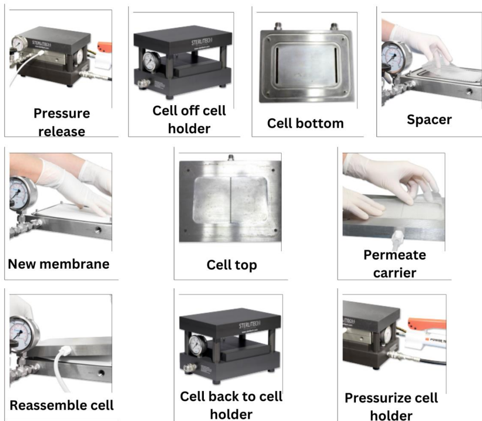
Figure 3-3: Membrane replacement (Sterlitech Corporation, 2017)
