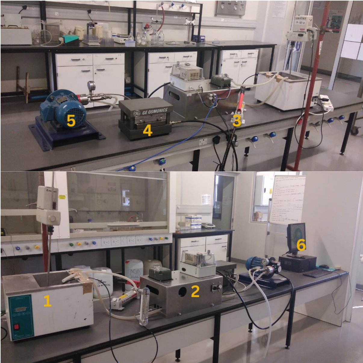
Photo 3-1: RO bench-scale system in the Environmental Engineering Research Laboratory (September 2022)
