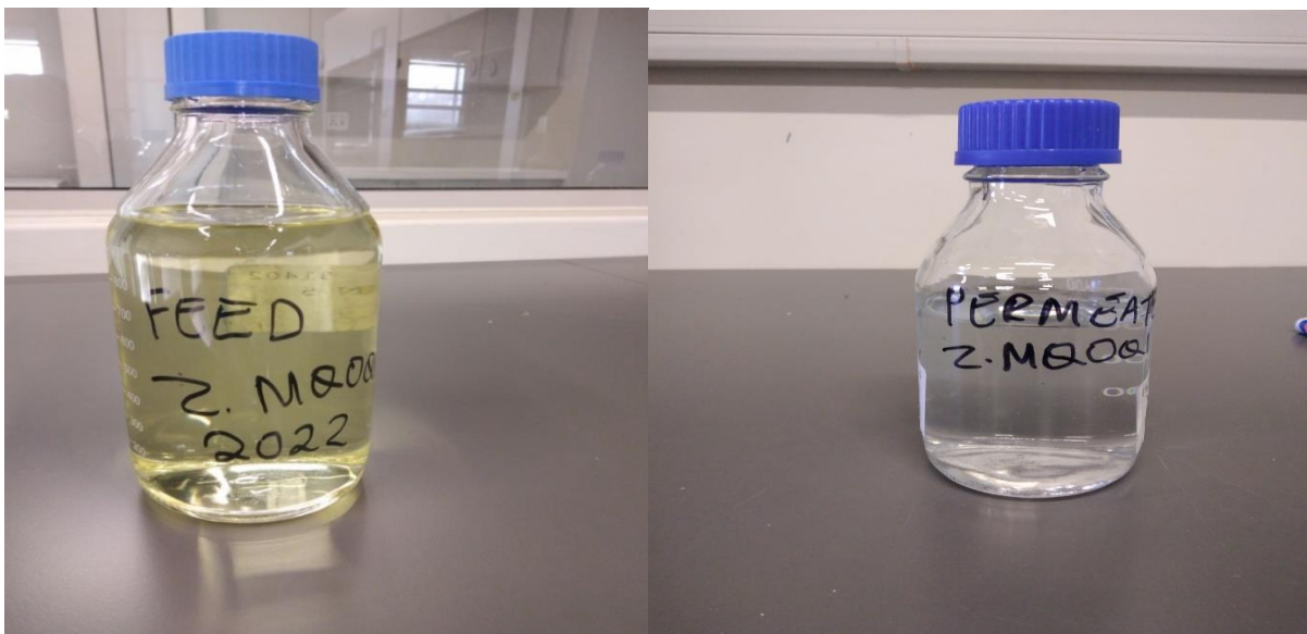
Photo 3-3: Synthetic MBR effluent (left) and permeate (right)
