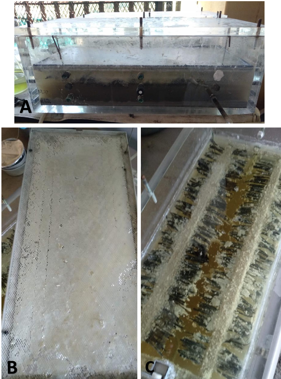
Figure A-3: Photographs of (A) Hybrid linear floor channel reactor, (B) Floating sulfur biofilm accumulated on the mesh screen and (C) colonisation of carbon microfibers in the bulk liquid
