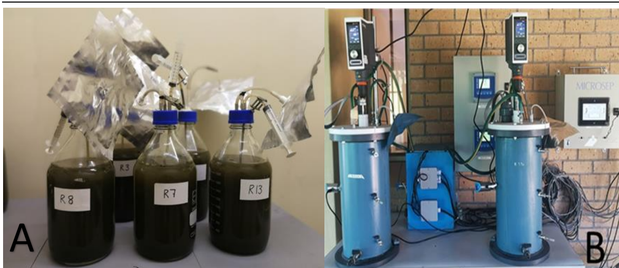
Figure 3-1: Set up of bioreactors for biochemical methane potential tests (A) and anaerobic sequential batch reactors, and related control systems (B))
