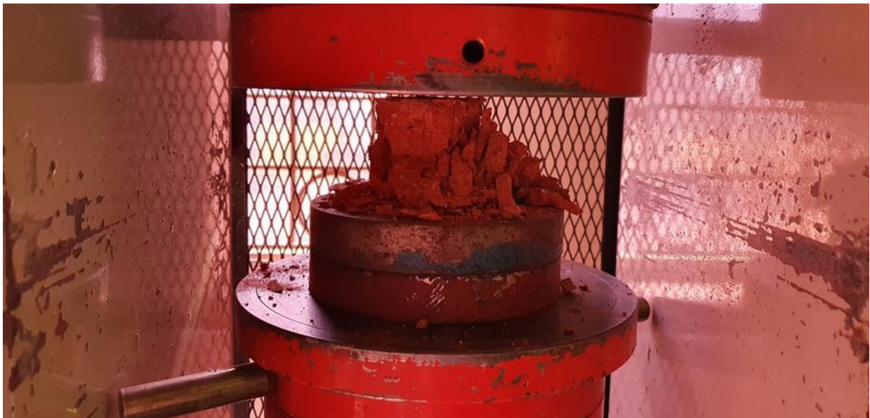
Figure 4.5: Crushed masonry brick sample
