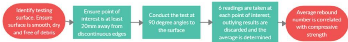
Figure 2.5: Rebound hammer test procedure (Rebound hammer test on concrete, 2018)
