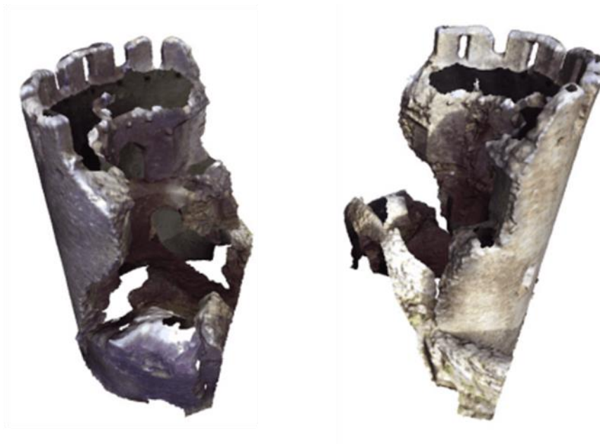
Figure 2.28: TIN mesh of the leaning tower developed from the laser scanning (D'Altri et al., 2018)
