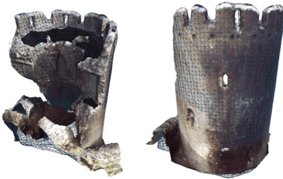
Figure 2.29: Finite element mesh superimposed on the TIN mesh of the leaning tower (D'Altri et al., 2018)
