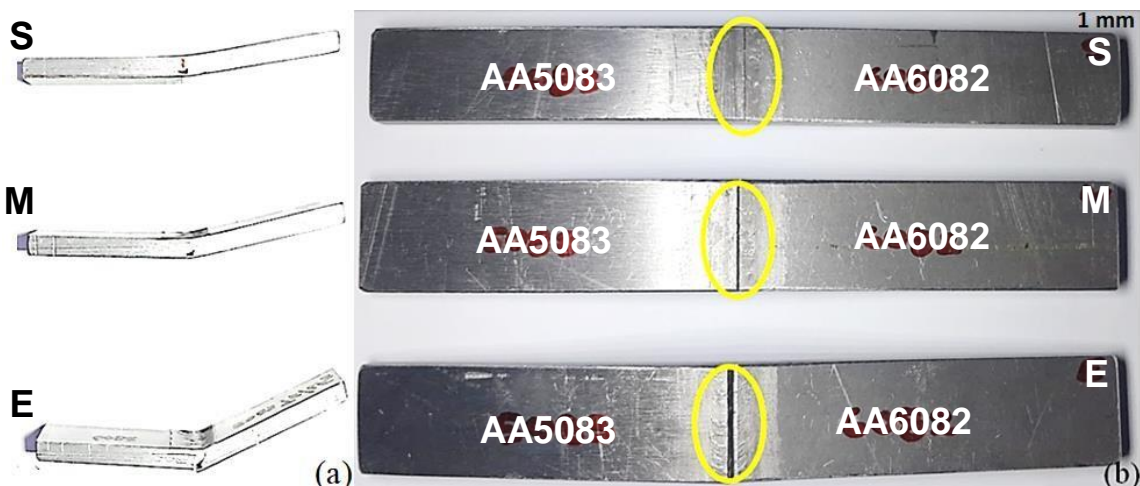
Figure 4.17: Root tested traverse samples (a) bent extent results and (b) surface and crack location results
