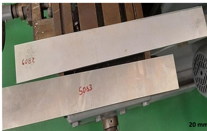
Figure 4.1: AA5083 and AA6082 blank materials
