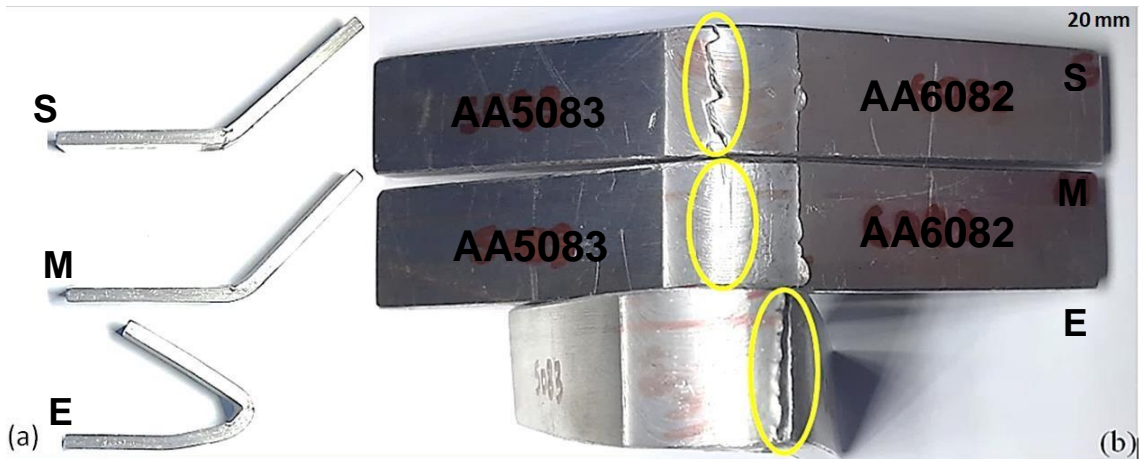
Figure 4.13: Face tested traverse samples (a) bent extent results and (b) surface and crack location results
