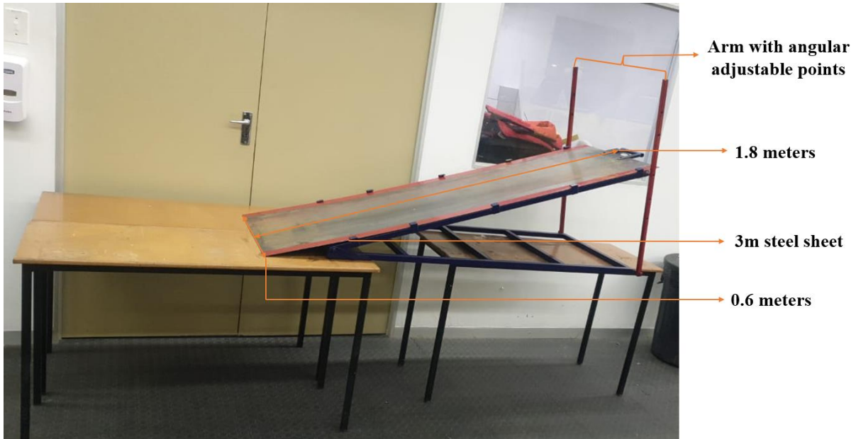
Figure 3.24: final design for the ramp describing the function
