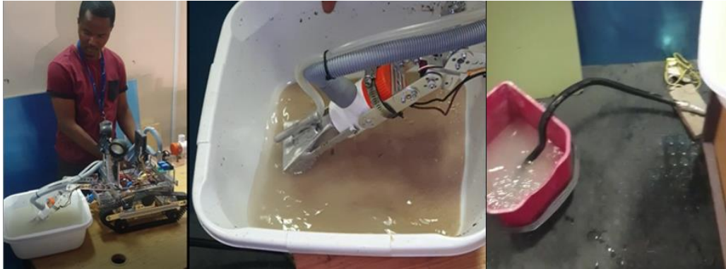
Figure 4.6: dredging sand sediment from a lower to higher region
