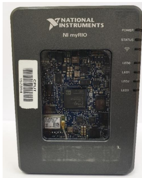
Figure 3.5: NI myRIO used for the control system of the EPRSDC
