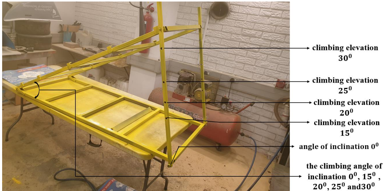
Figure 3.23: structural frame of the test ramp
