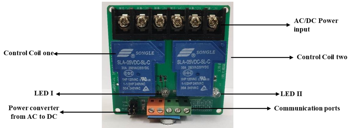
Figure 3.15: 12–240-volt relay module used in controlling the dredging and jet pump system of the EPRSDC
