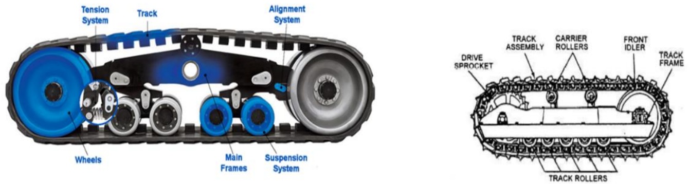
Figure 2.31: fundamental parts of a robotic track drive system (Daanen, 2017)
