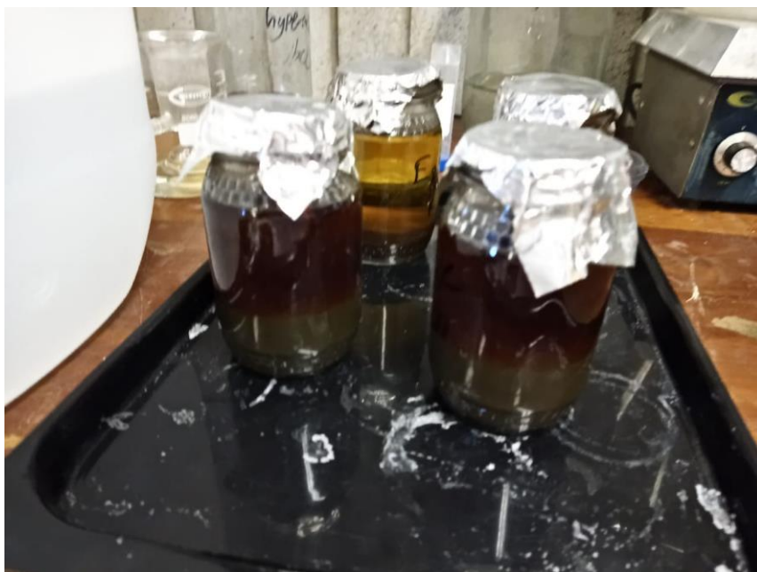
Appendix C-8: Dried sediments mixed with KOH and NaCl
