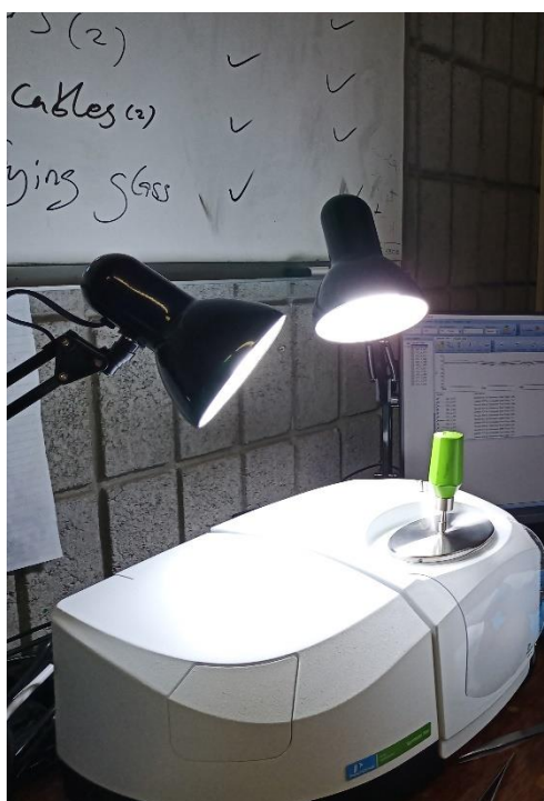
Appendix C-9: FTIR Instrument for polymer analyses
