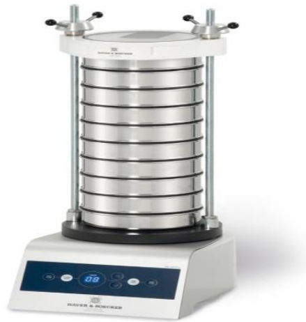
Figure 3. 4: Sieves of different mesh sizes on mechanical shaker.
