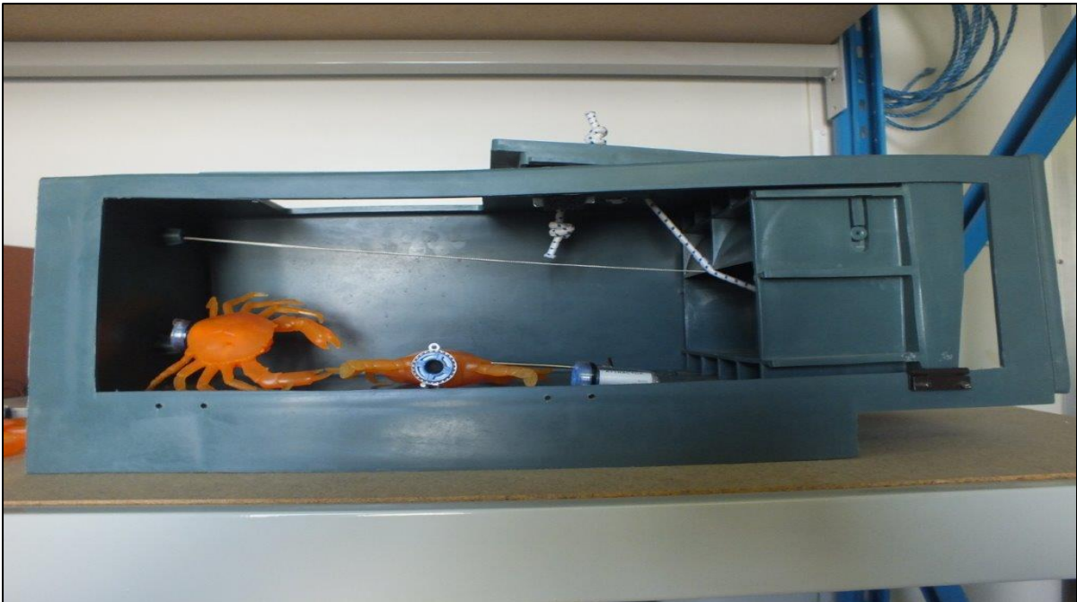
Figure 3.5: Cross-section of trigger trap shown in activated position
