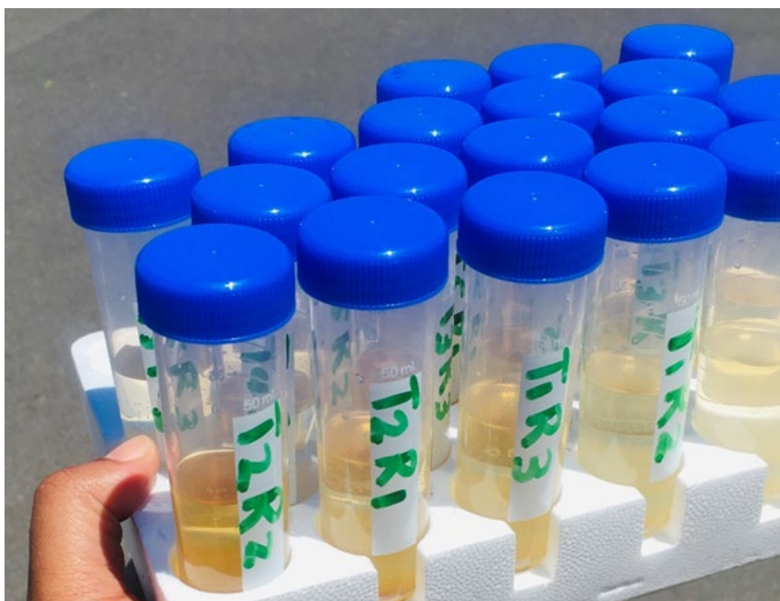
Figure 3.5 Centrifuge tubes containing mixture of powdered bulb plant material and 20 mL of solvent made up of 60% ethanol and 40% distilled water.
