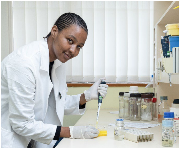
Figure 4.3: Pipetting a reaction mixture into test tubes during the determination of proline in C. subternata leaves.
