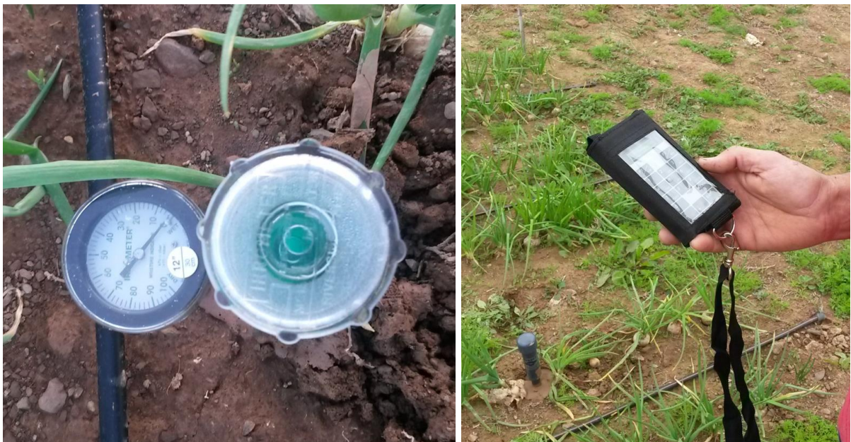
Figure 3. 9: Tensiometer calibration and setup of data collection software for Probes.
