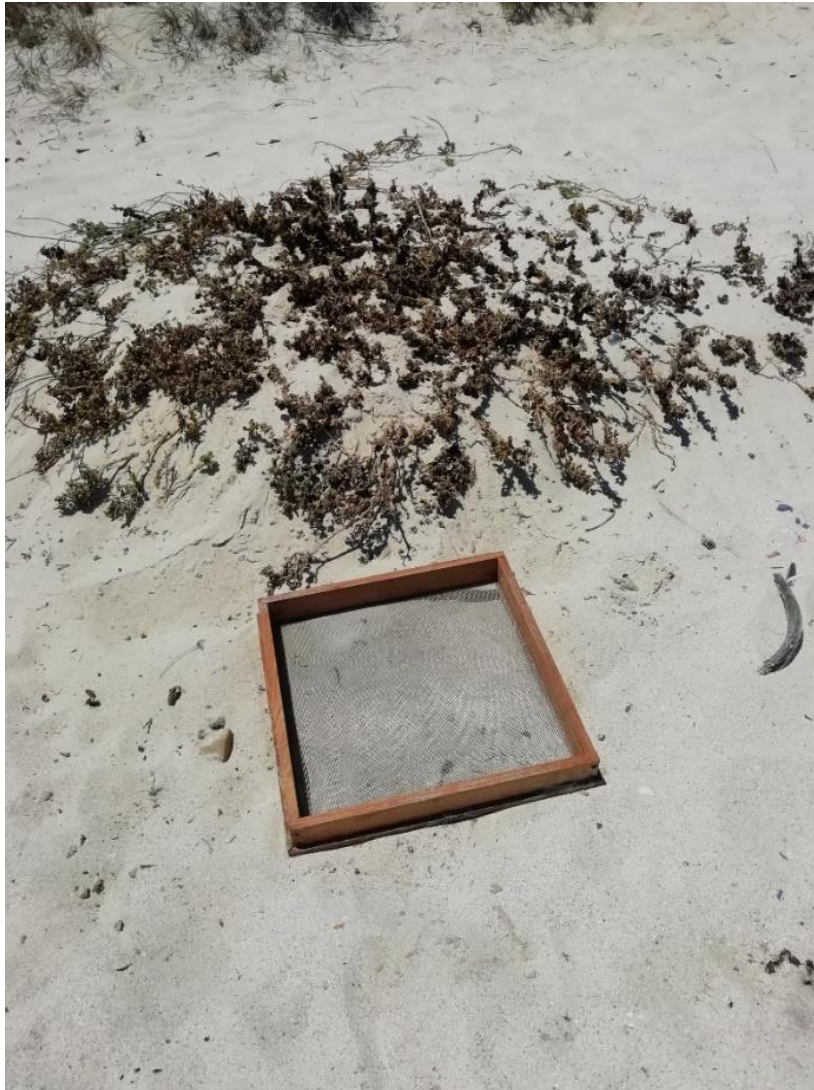
Figure B. 3: A 0.5mX0.5m sieve with 2mm mesh used for the collection of mesolitter
