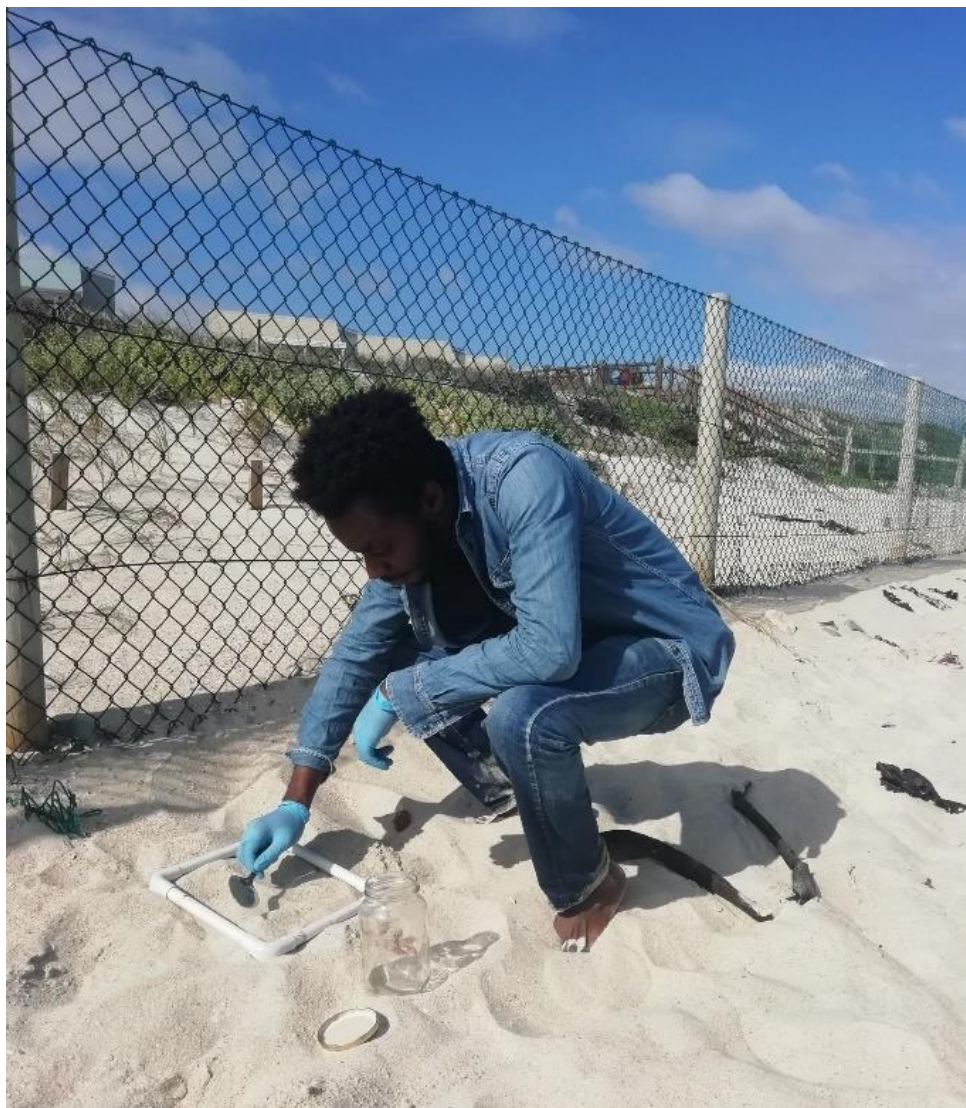
Figure B. 1: Collection of sediment samples from the backshore for MPs analysis
