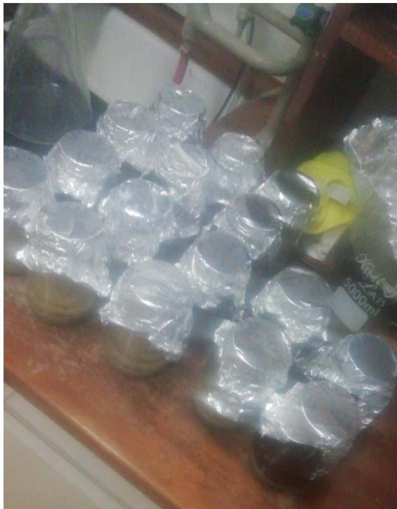
Figure D. 1: Digestion of sediment samples with 10% KOH solution
