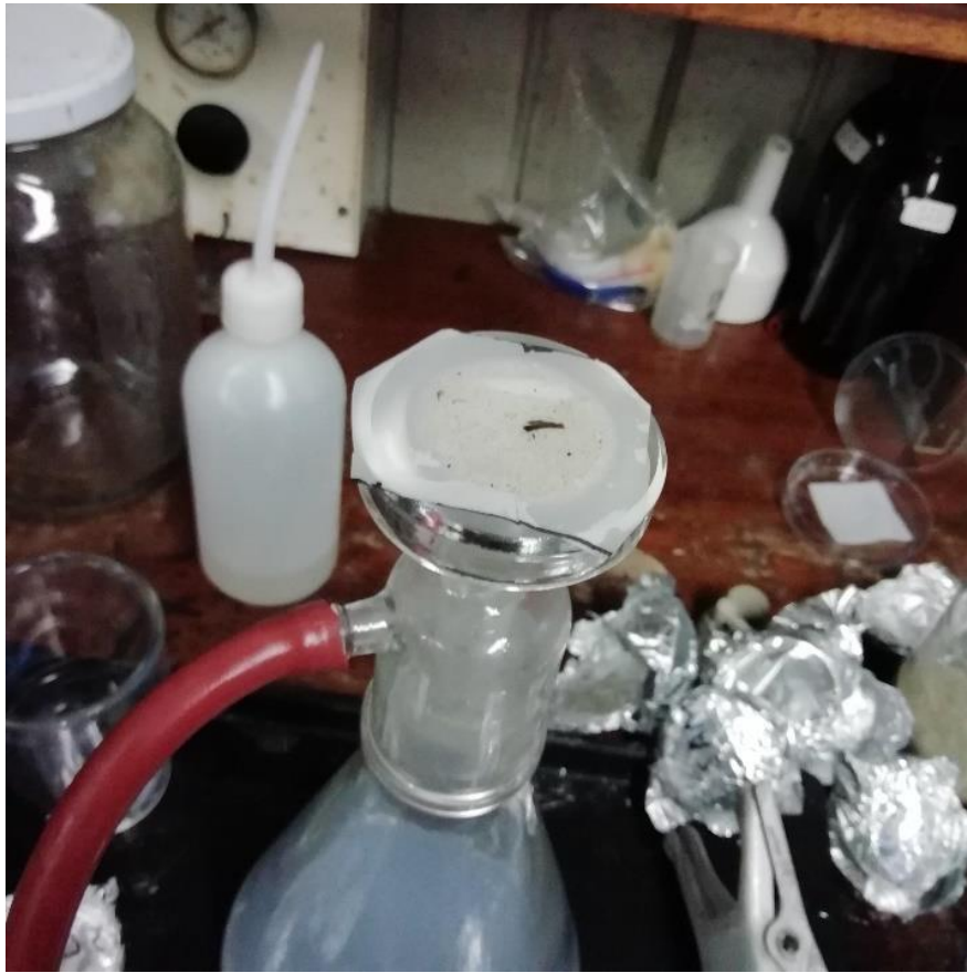
Figure D. 2: Filtration of samples through a 20 \mu\text{m} mesh for microplastic extraction
