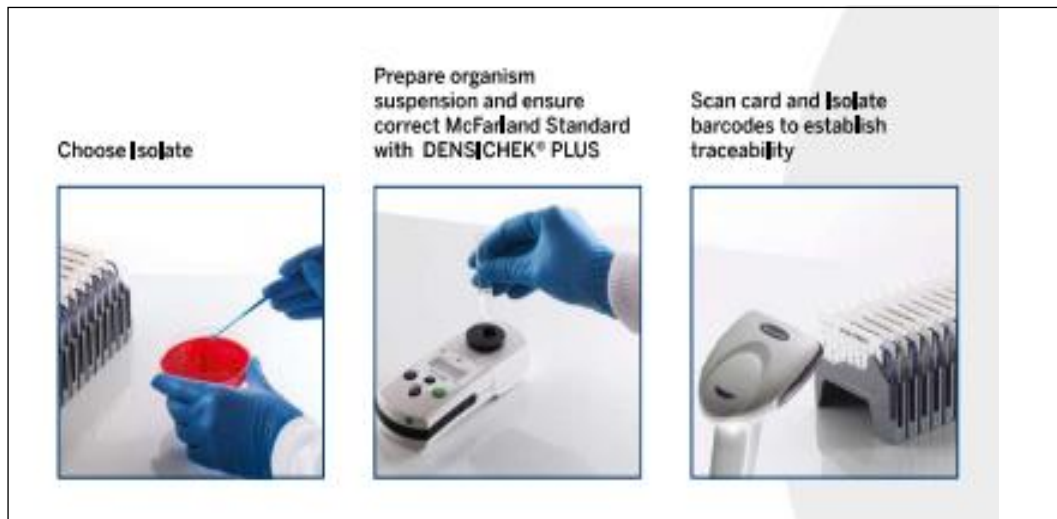
Figure 18: Loading the VITEK® 2 system with a bacterial suspension
