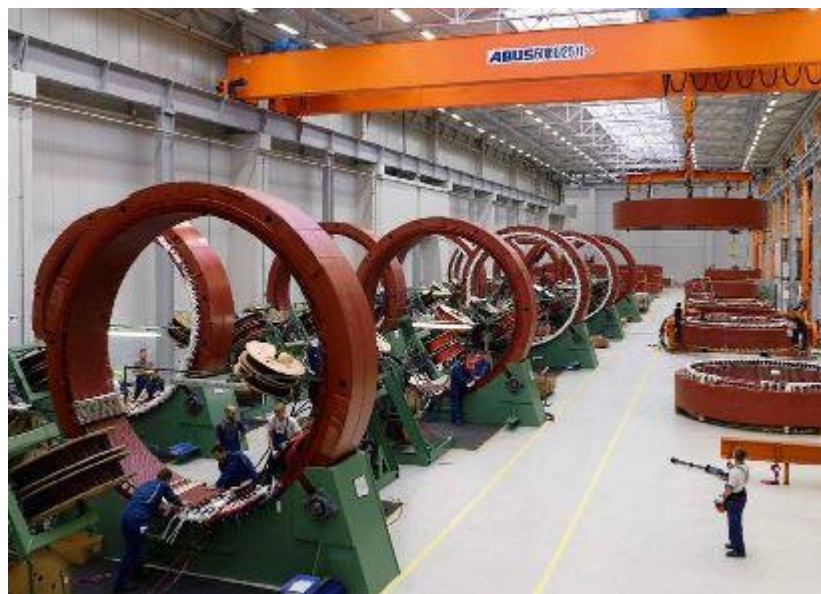
Figure 1.4: Annular generator manufacturing at Enercon, Magdeburg, Germany
