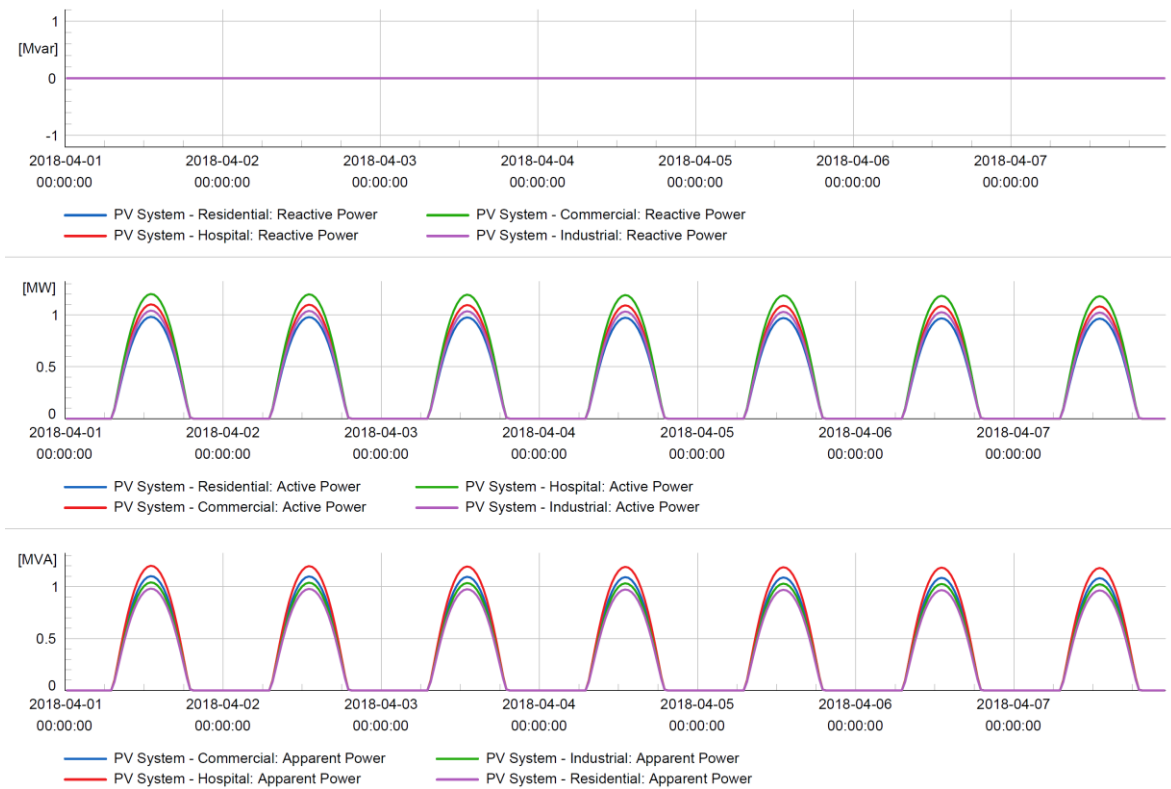
Figure 6-7: PV output curves
