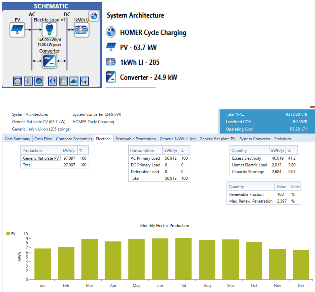
Figure 23: Homer connection of solar for compressor only.
