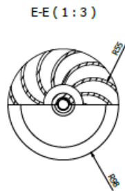
Figure 16. Water impeller, sectioning view
