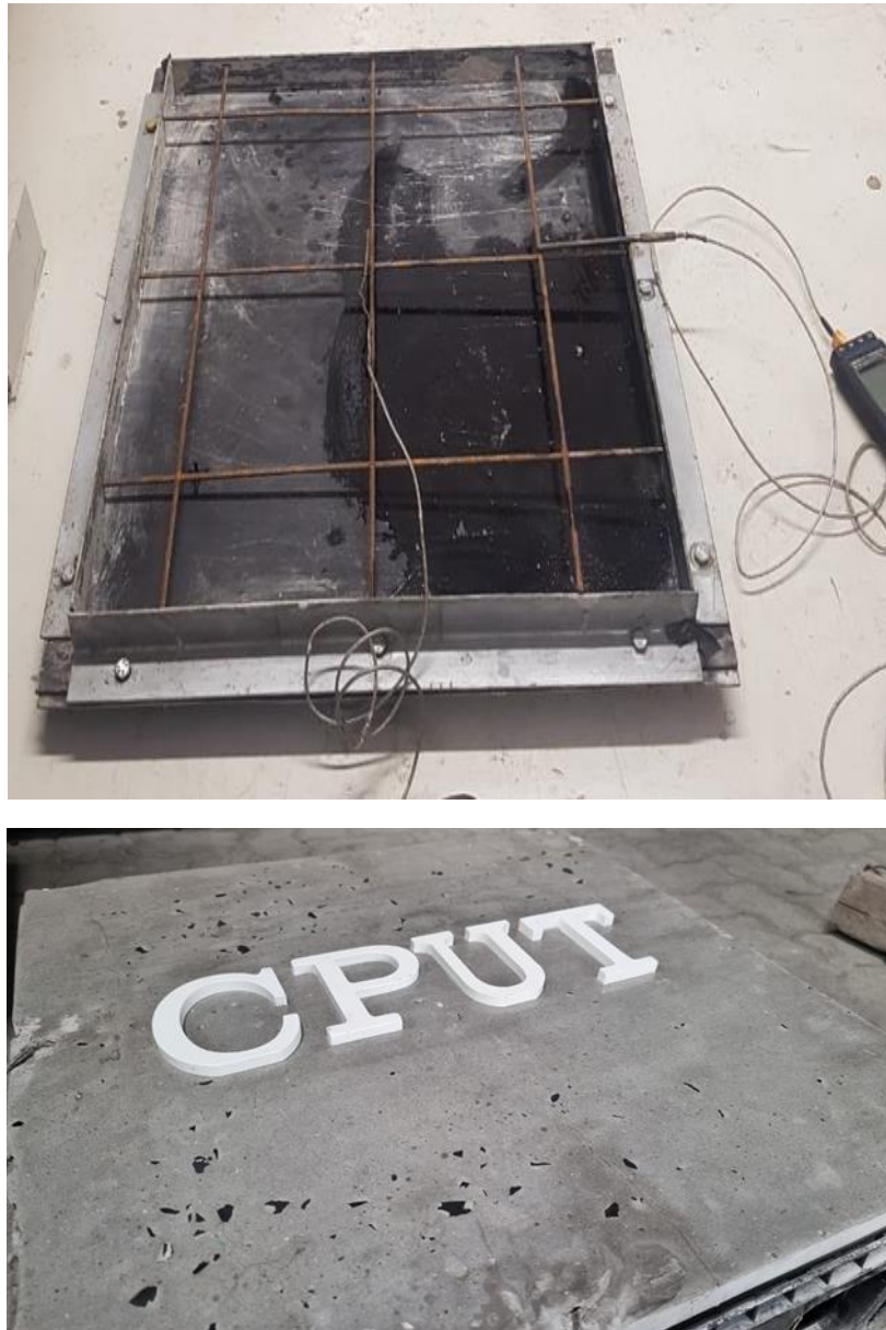
Figure A-8: Fire test sample mould with Y6 reinforcement steel (a) and fire sample after finished (b).
