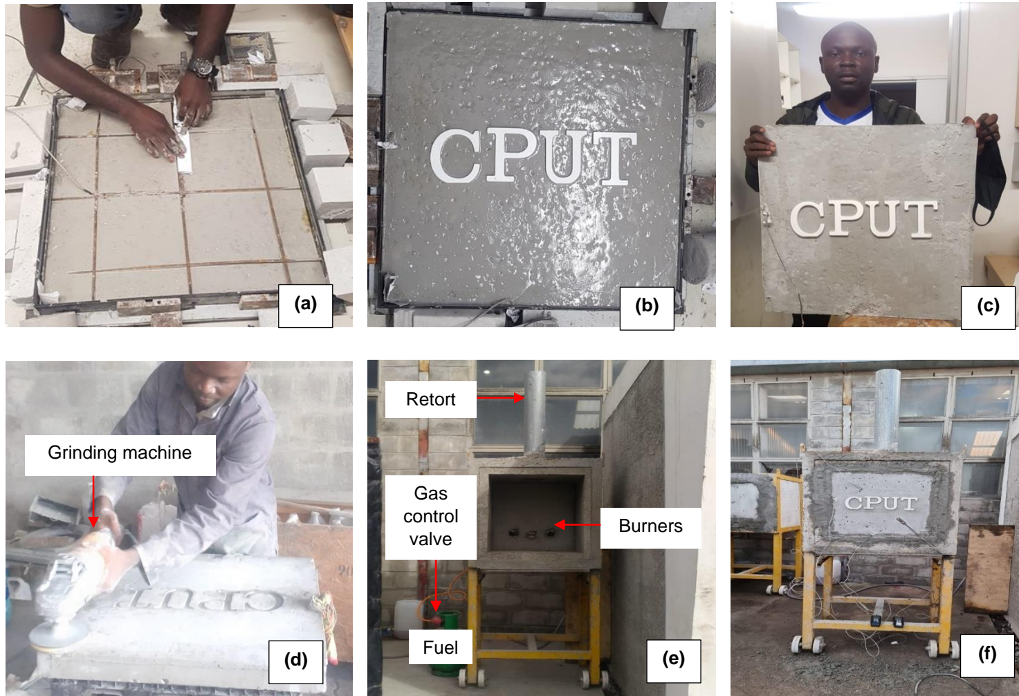
Figure 3-29: Steps involved in casting to the testing of low calcium CFA-based geopolymer reinforced concrete; panel being cast and steel reinforcement after bottom the casting of the bottom cover (a), Panel at the end of casting (b), demoulded panel after three days of ageing (c), grinding and polishing of the panel in progress (d) and NES Consult 600x600x60 designed fire oven used for testing (e) and panel oven installation ready for fire testing (f)
