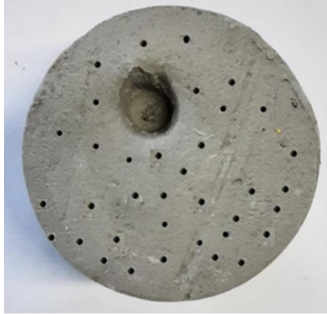
Figure A-10: CFA-based geopolymer paste after Vicat apparatus test
