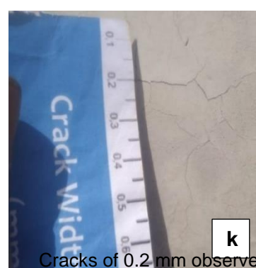
Panel fire exposed surface at the end of the test (E) Page 153 of 270
