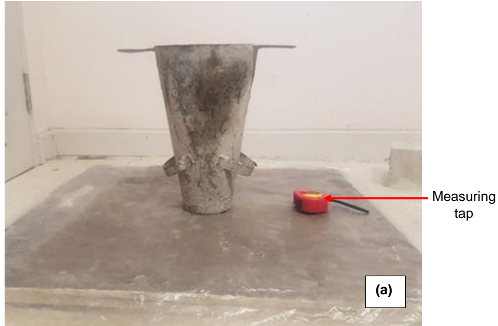
Figure 3-16: Slump flow apparatus and wet CFA-based geopolymer concrete during slump flow test.
