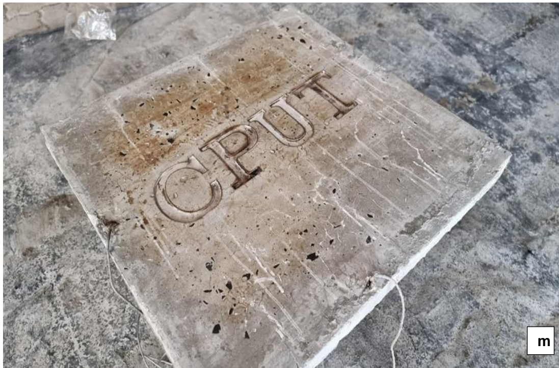
Unexposed surface of the panel after being demoulded from fire oven (U)
