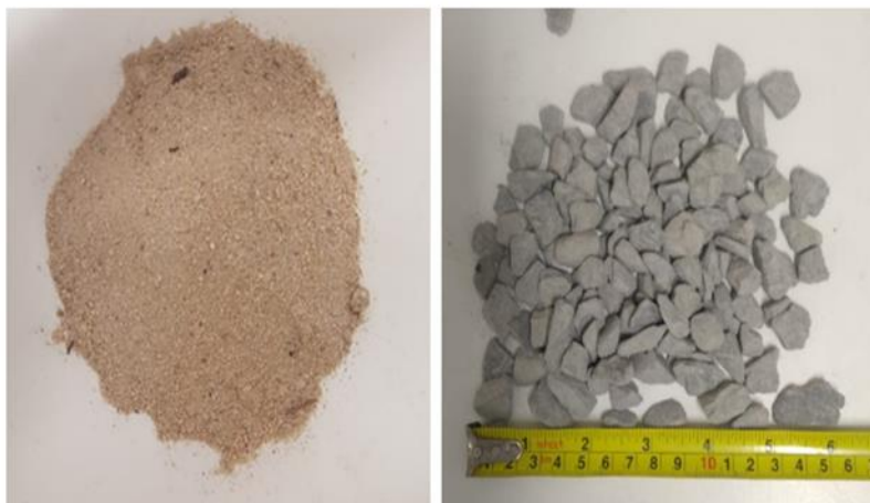
Figure 3-2: Philippi used as fine aggregate (a) and blue stone as coarse aggregates (b) for the synthesis of CFA-based geopolymer mortar and concrete.
