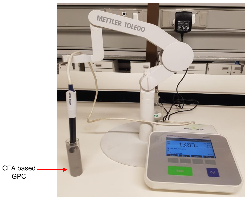
Figure 3-26: Lethabo low calcium CFA-based geopolymer concrete at fresh state pH measurement in progress.
