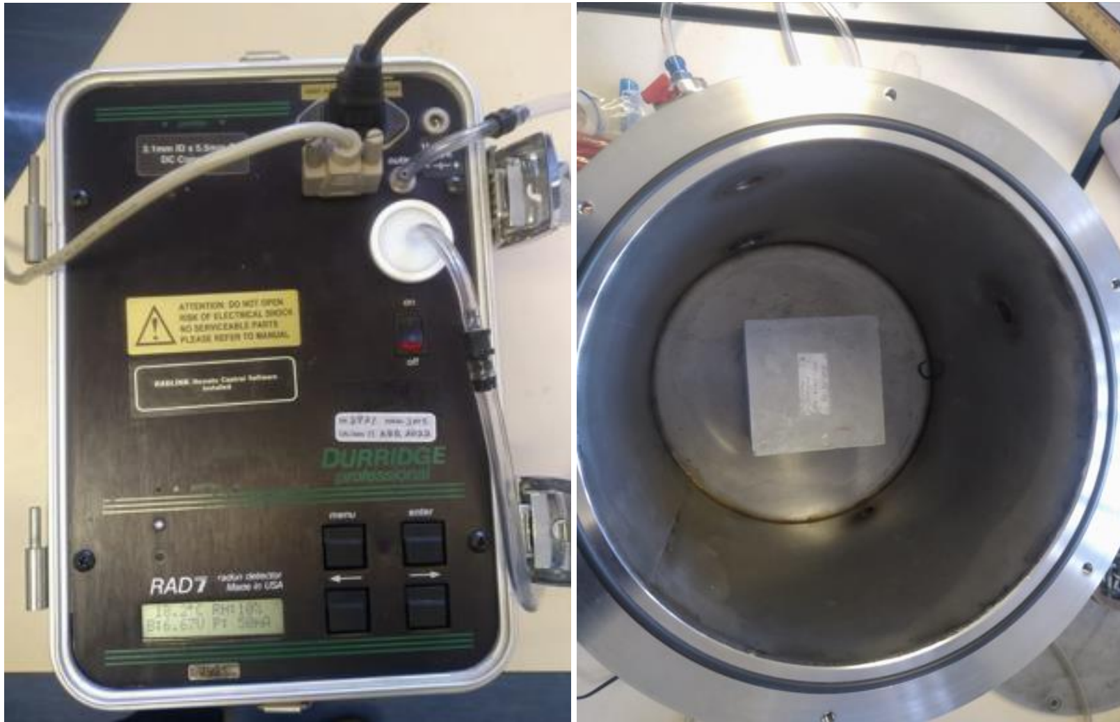
Figure A-9: Top face of radon measurement RAD 7 (a) and 100 mm cubic CFA-based geopolymer paste block inside a gamma vacuum chamber.
