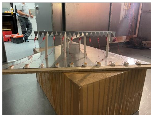
Figure 6.16: Photograph of DUT flat on ground plane of the conical terminated TEM cell, SARAO facilities
