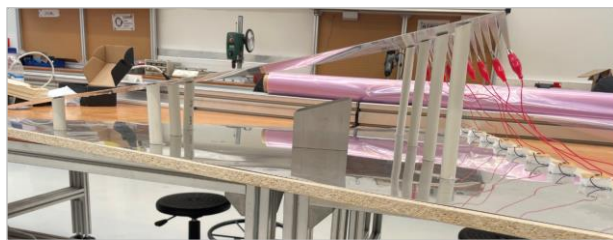
Figure 5.5: Picture of DUT inside cell with centre at 635 mm from feeding SMA connector
