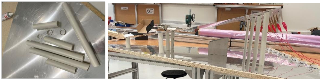
Figure 4.19: Cut PVC pipe plate (left). Photograph illustrating cut PVC pipe used to support top plate (right)
