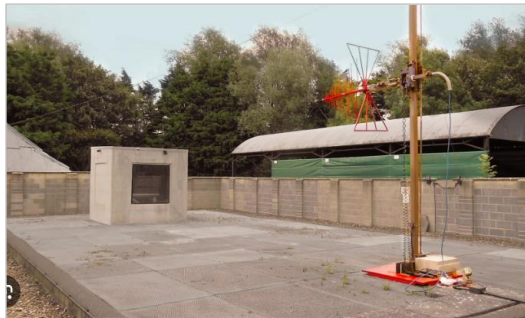
Figure 2.4: A low level swept field OATS setup (Intel Platform Design).
