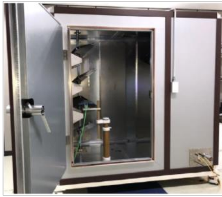
Figure 2.1: Picture illustrating reflective surfaces and stirrers inside a reverberation chamber (Sim et al., 2019)
