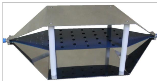
Figure 2.8: Photograph of a conventional TEM cell (emcsupplies.com, n.d)
