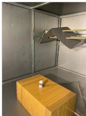
Figure 6.9: Picture of Comb Generator in reverberation chamber at SRAO facilities.
