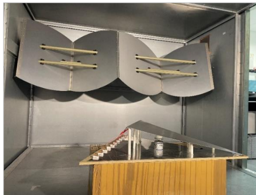
Figure 6.12: Comb generator housed inside conical terminated TEM cell and inside reverberation chamber at SARAO.
