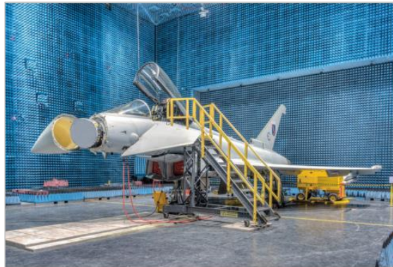
Figure 2.3: Semi-anechoic chamber at an Electronic Warfare Test Facility (Pywell & Midgley-Davies, 2017)
