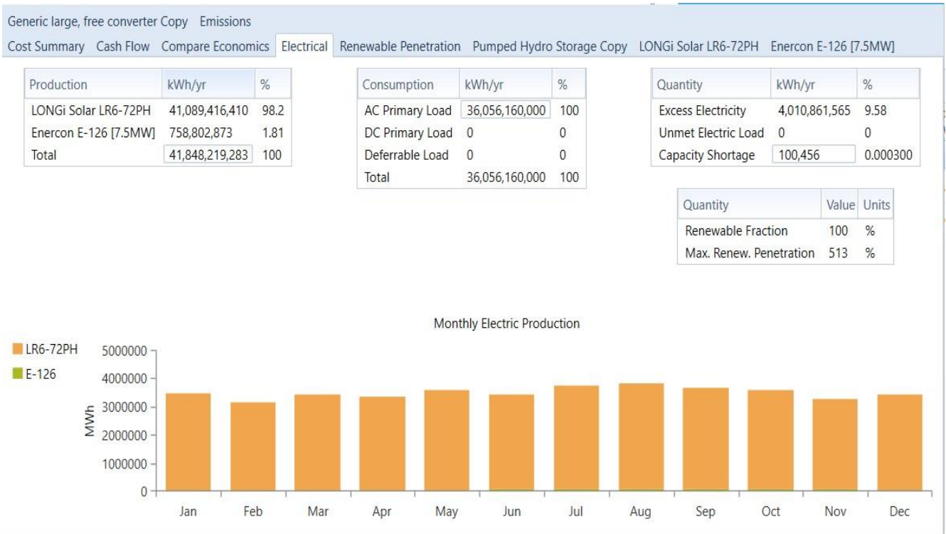
Figure 5.7.2.2.1: The electrical results obtained from HOMER Pro for the second system of the optimizer process
