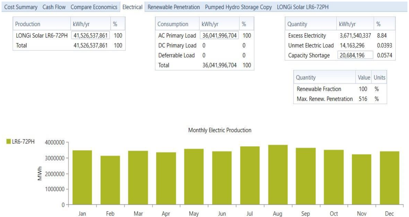
Figure 5.7.2.1.1: The electrical results obtained from HOMER Pro for the first system of the optimizer process
