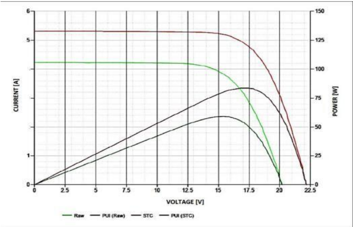
Figure 3.3.1.1.3: The current, voltage and power curve of a monocrystalline solar PV panel at high irradiance. [21]
