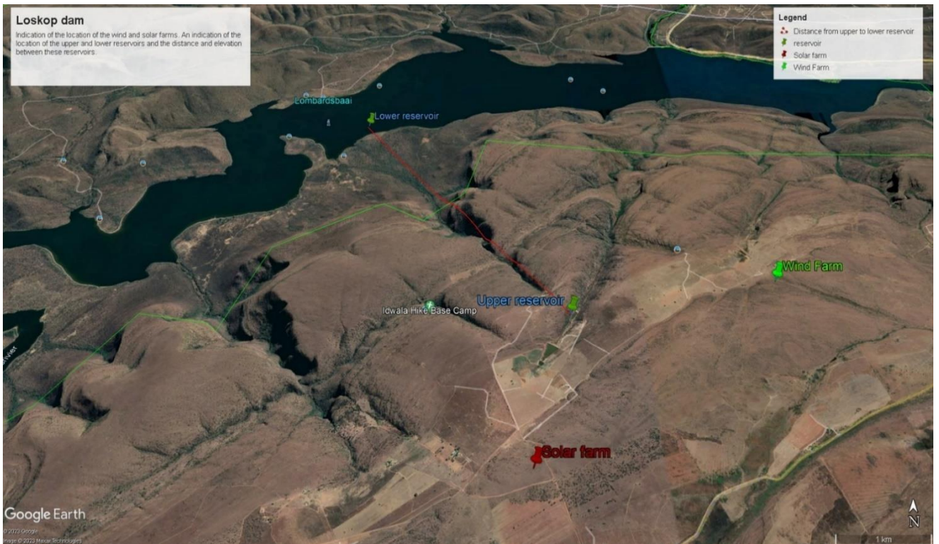
Figure 4.2.2.2: An indication of the location of the proposed HRES system near the Loskop Dam. This figure indicates the wind and solar PV system and the upper and lower reservoirs for the pumped hydro storage system.
