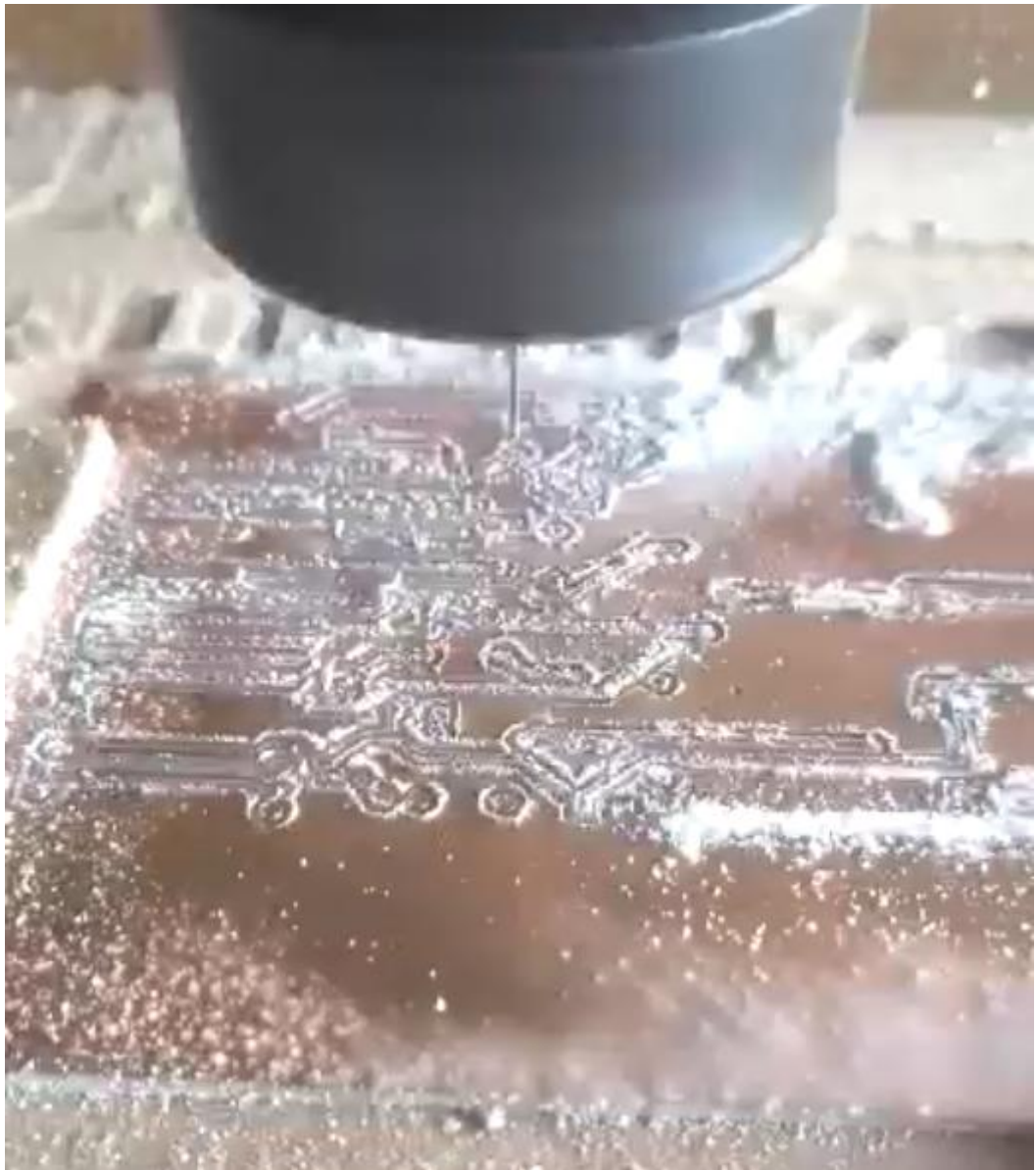
Figure 3.15: Milling of the controller board PCB
