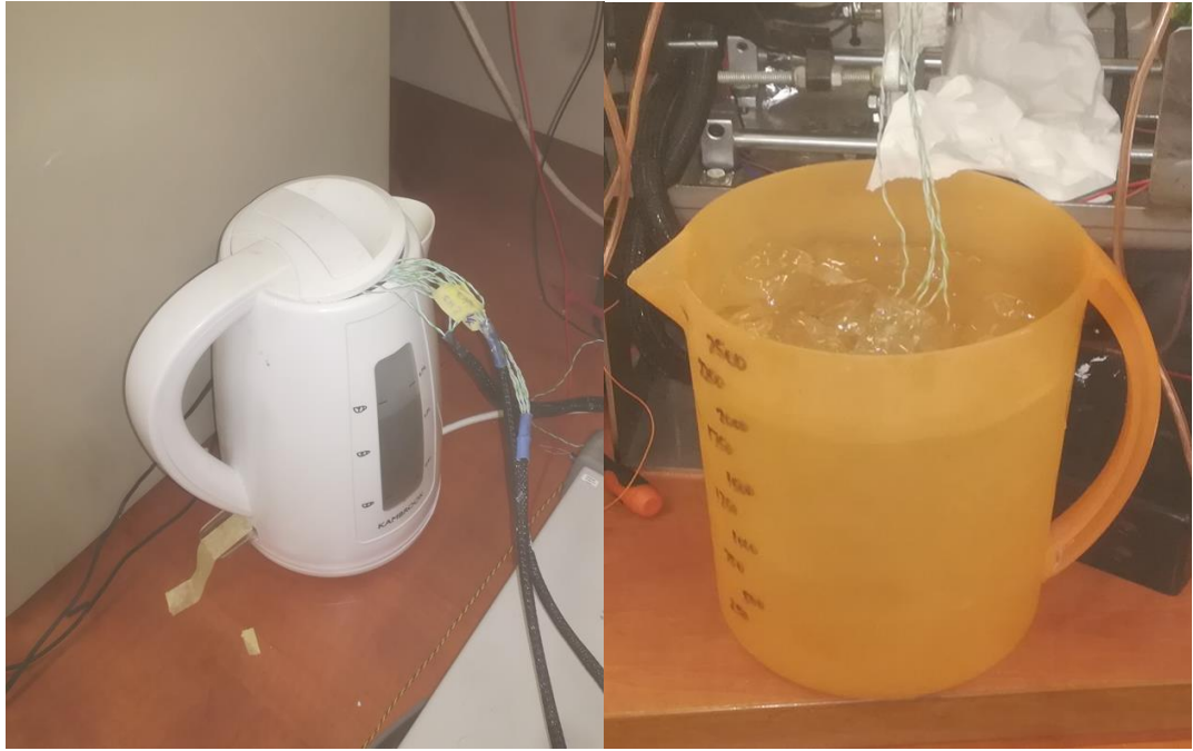
Figure 4.1: Left: cold temperature calibration; Right: hot temperature calibration
