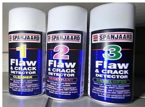
Figure 3.6.3: Liquid penetrant 3-step spray cans.
