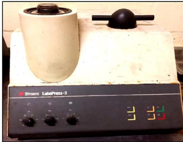
**Figure 3.3.2: Struers Labopress 3 machine.**
