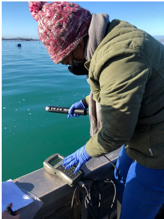
Figure 6 Documenting temperature and pH readings with a multimeter
