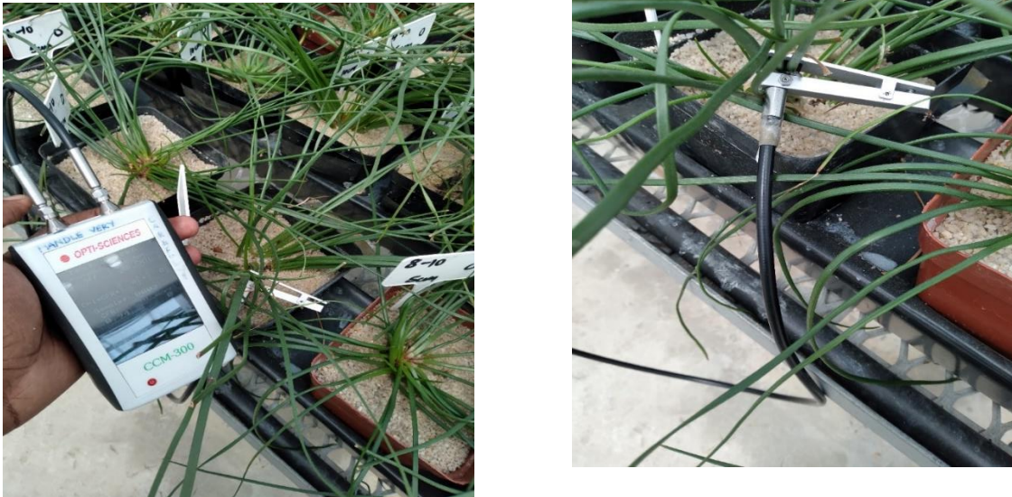
Figure 4.5.1: Collection of chlorophyll on three leaves that were marked specifically for chlorophyll data (Bulawa, 2021).
