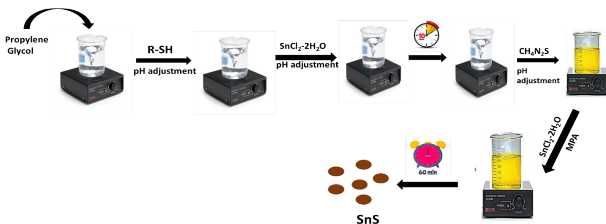
Figure 3.2. Schematic representation of SnS QDs (method 1).
