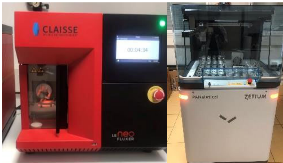
Figure 3.18 The XRF Claisse LeNeo fusion and PANalytical Zetium compact spectrometer
