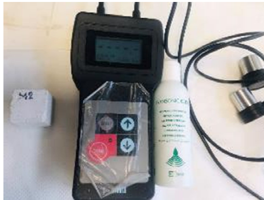
Figure 3.21 The UPV tester used to test mortar compactness using transducers with 54 kHz frequency on three perpendicular sides of 40 mm 3 cube mortars
