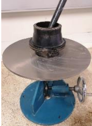
Figure 3.10 Fresh mortar workability testing using a flow table test
