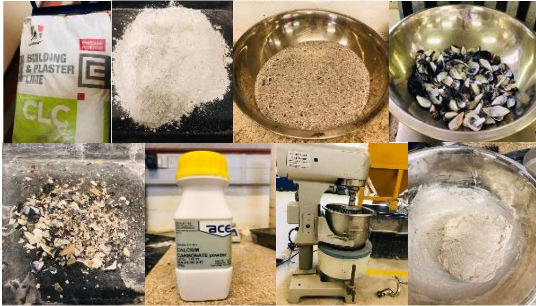
Figure 3.9 Raw materials (from left to right): hydrated lime, sea sand, seashells and calcium carbonate and mixing procedure for new mortars using both machine mixing and hand mixing
