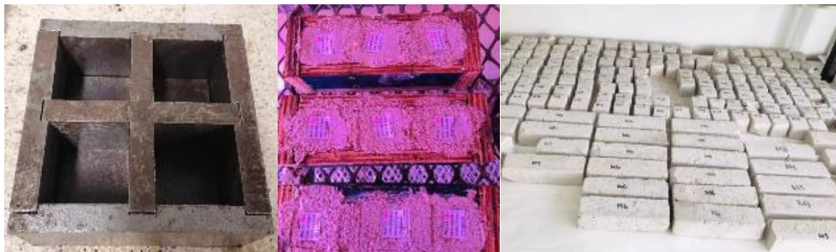
Figure 3.11 Mortar cubes preparation, casting, demoulding and curing procedure
