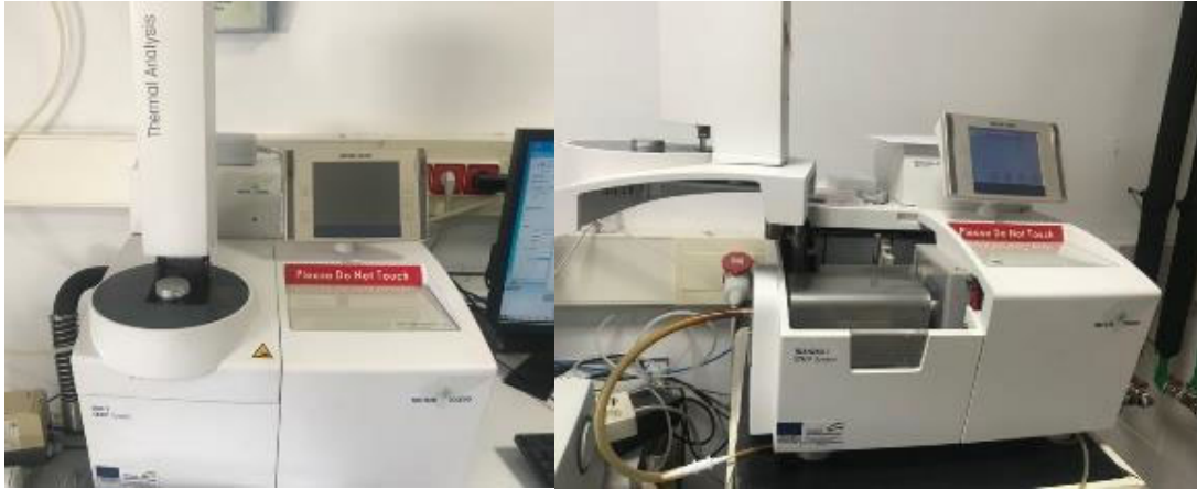
Figure 3.20 The TGA/DSC 1 HT/851 DIC-2021-2 instrumentation for analysing the thermal weight loss of binder content in mortars
