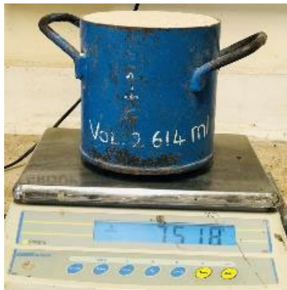
Figure 3.8 Determining the densities of aggregates using SANS 3001-GR6, Part 6
