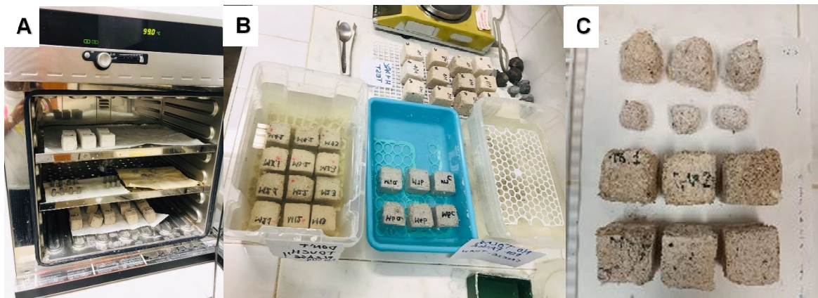
Figure 3.13 Samples during salt crystallisation cycles demonstrating A) Drying of samples at 100°C B) Immersion in deionised water and C) Change in weight and shape over the 15 cycles
