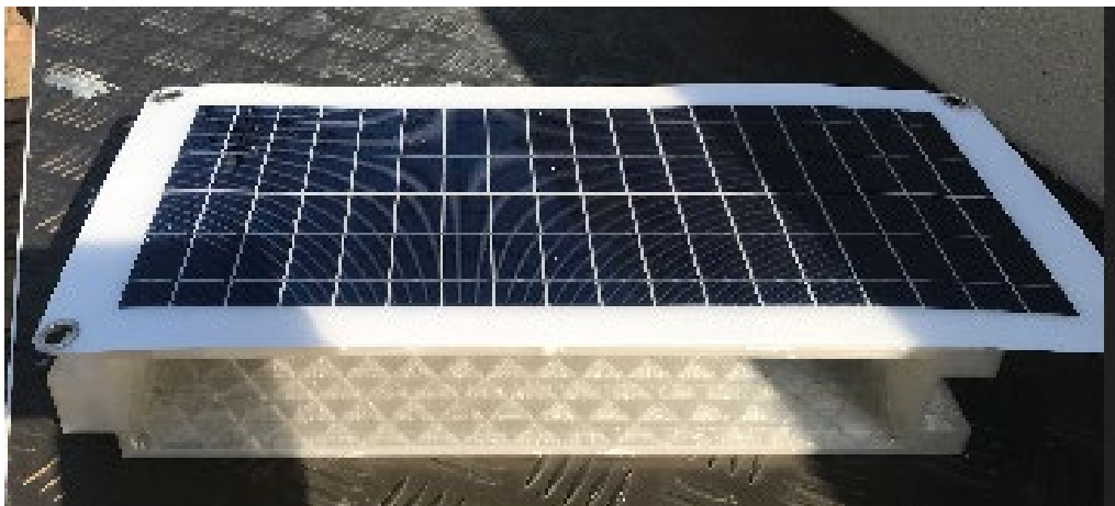
Figure D.6 Model: Prototype building panel showing rainwater tank, building panel and FSC
