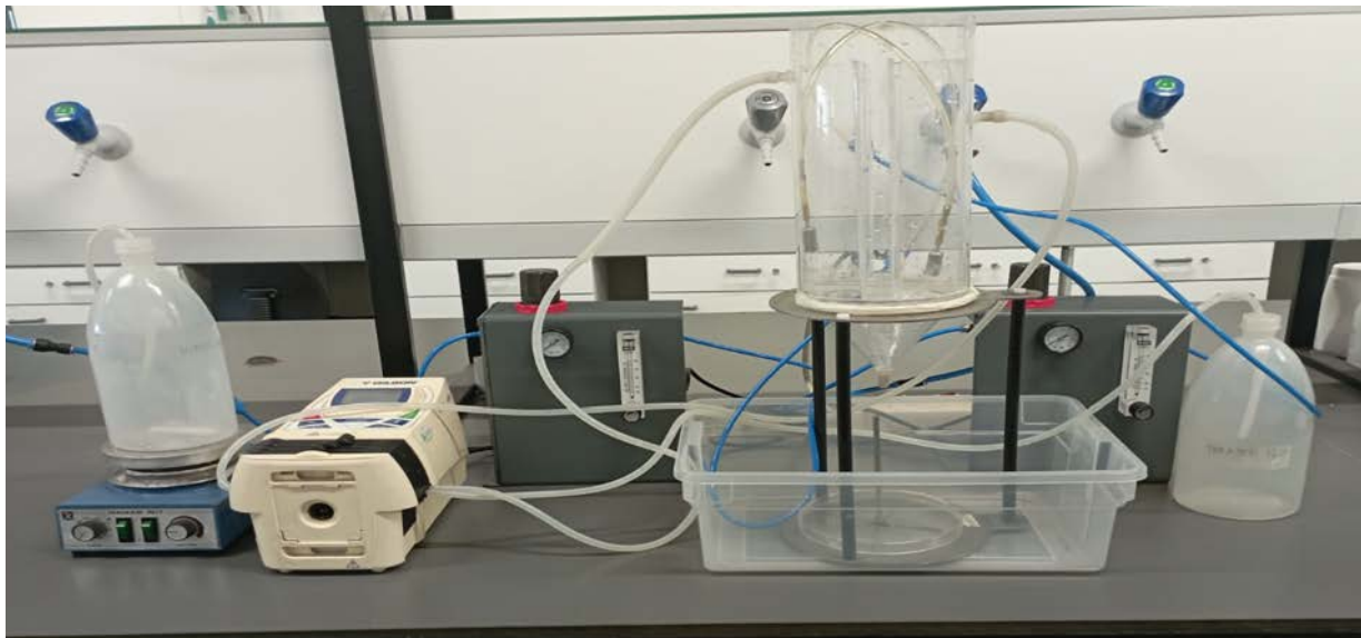
Figure 12: Photographic illustration of a column flotation.
