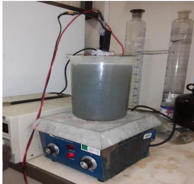
Figure 3. 1: Electrocoagulation experimental set-up
