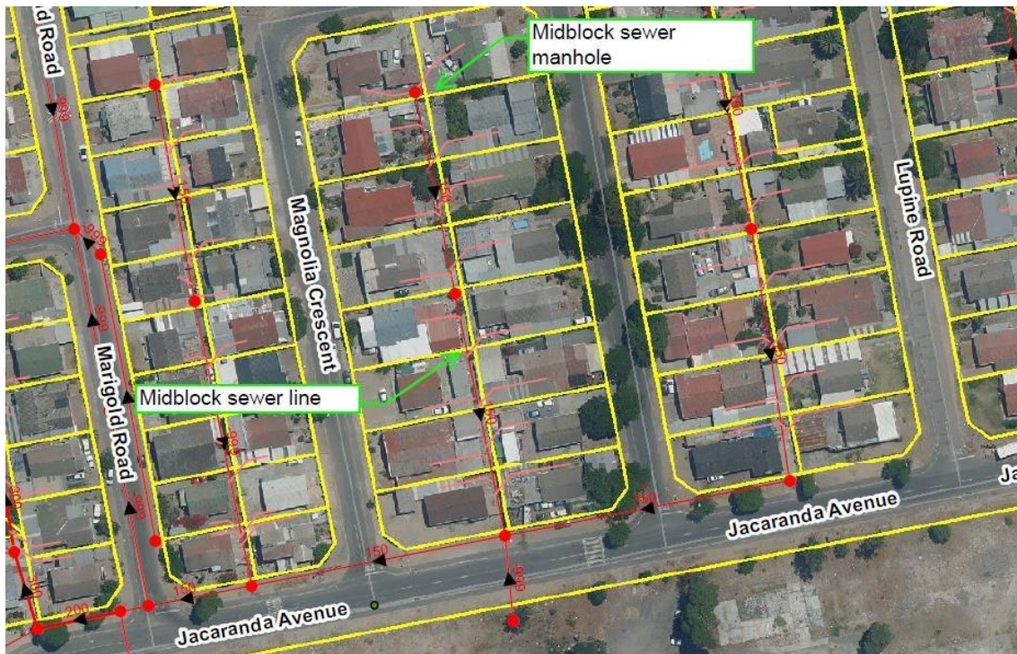
Figure 4.16: Illustration of midblock sewer line ( Source: City of Cape Town GIS Viewer)
