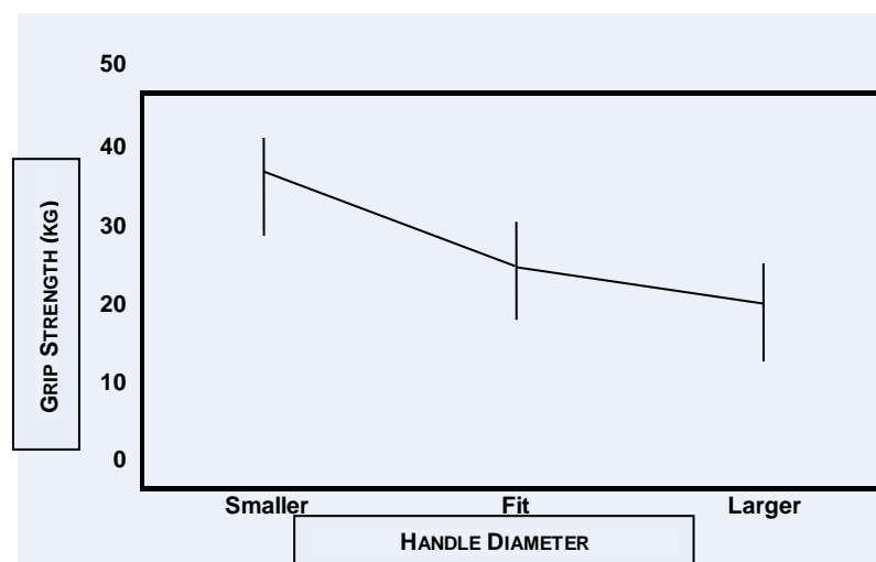
Figure 2.9: Maximum grip strength as a function of handle diameter (Grant et al. , 1992)
