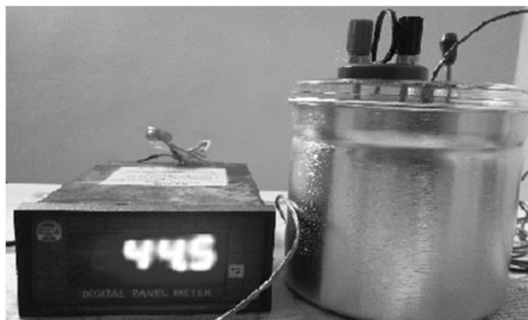
Figure 2.17: Thermal conductivity set up for \text{Co}_3\text{O}_4 -DI water nanofluids (Sekhar et al., 2017)
