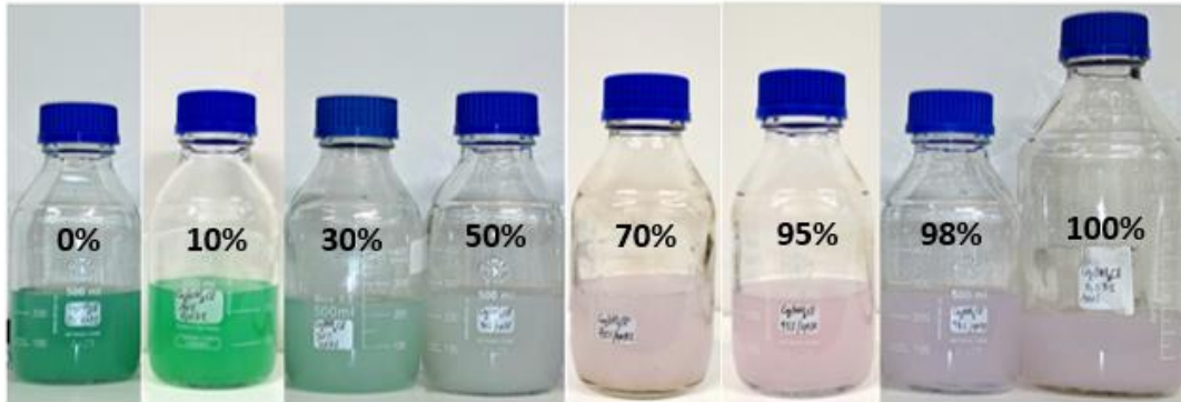
Figure 3.5: \text{Co}_2(\text{OH})_3\text{Cl}-\text{H}_2\text{O} nanofluids produced from different propanol concentrations at 0.03 wt% after 4 h of sonication
