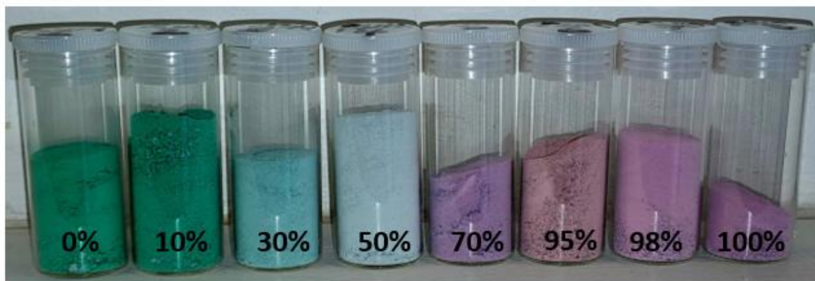
Figure 4.6: \text{Co}_2(\text{OH})_3\text{Cl} nanopowders at propanol concentrations ranging from 0 to 100% (left to right)
