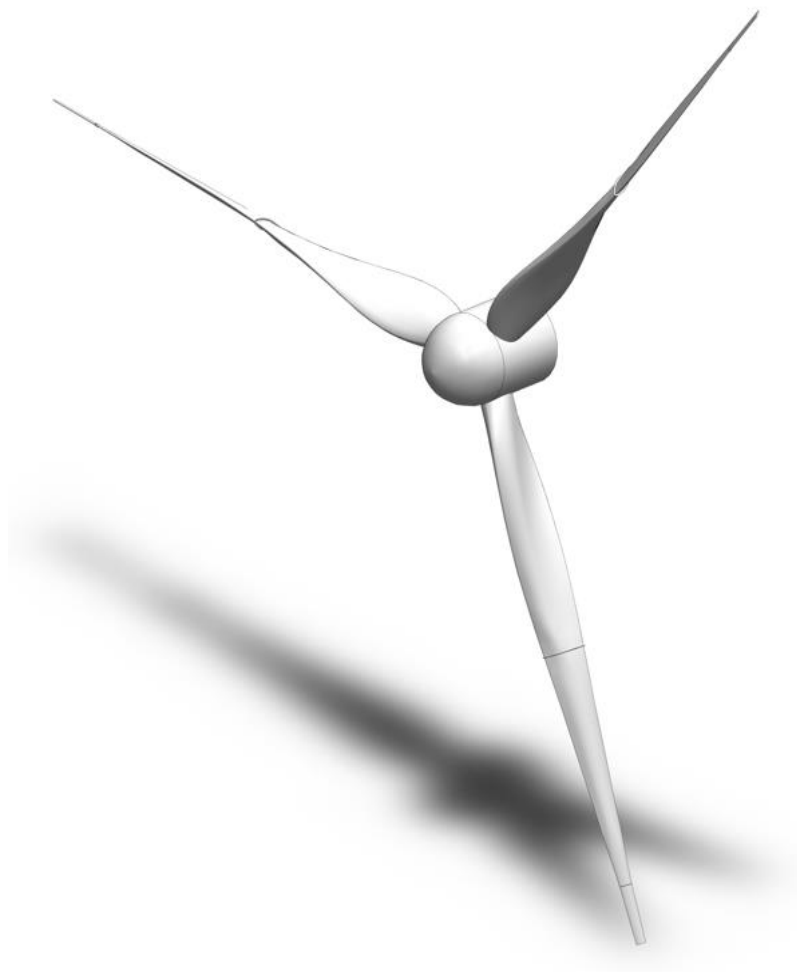
Figure 5-21 : NREL 400kW blade – Attached to a generic hub with fences at 50% and 90% of the full length of the blade. (Author’s work)
