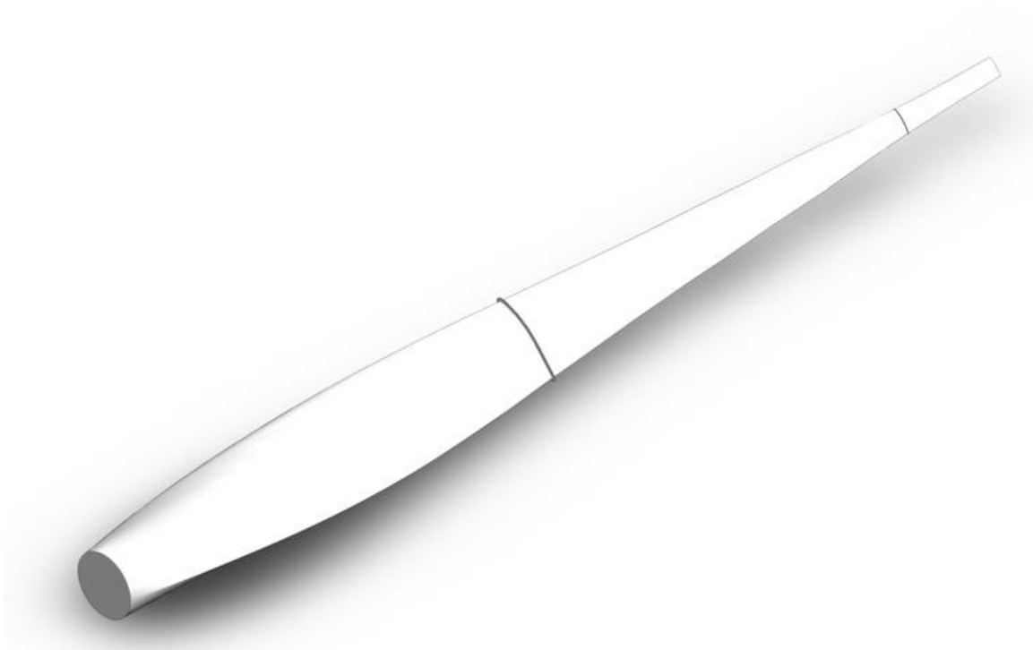
Figure 5-23 : NREL 400kW blade – Showing the full blade with 20% augmented fences installed as per the results of the fence height analysis. (Author’s work)
