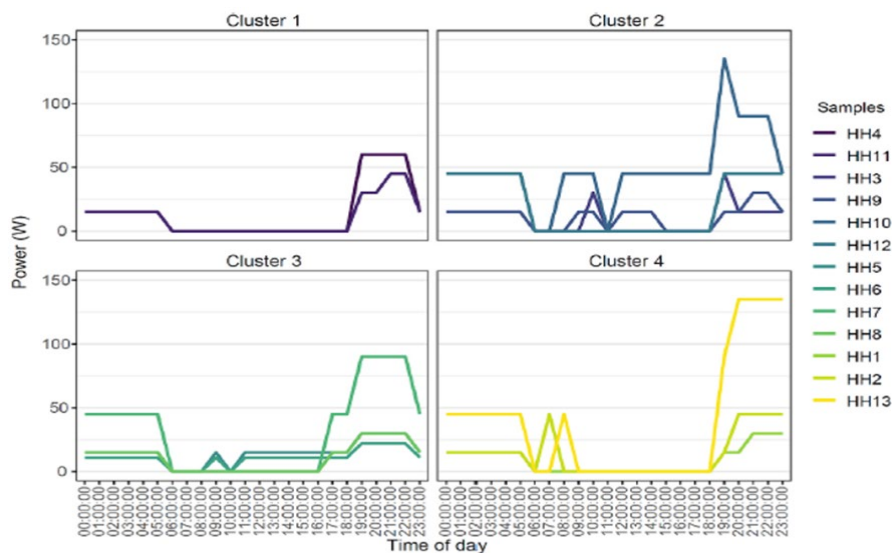
Figure 3-3: Results from the simulated lighting load profiles for households (HH) in each cluster (Dominguez, C. et al., 2021, p. 11).
