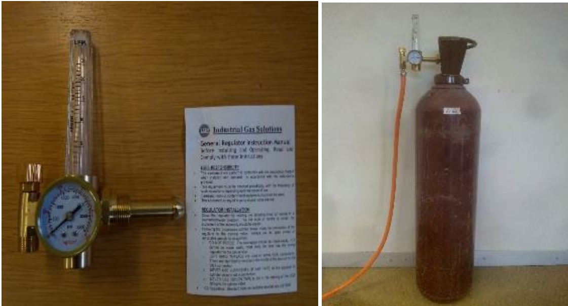
Figure 3-19: Industrial helium Gas regulator.
