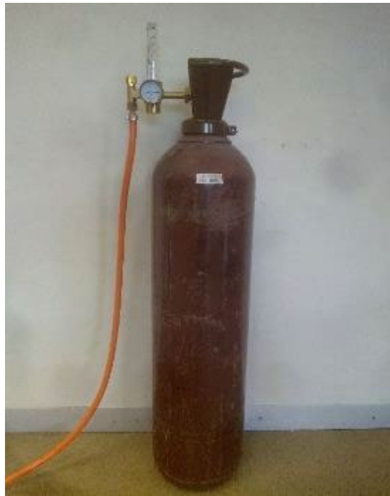
Figure 3-20: A cylinder of 20 litres pressurised with helium at 3000 PSI.
