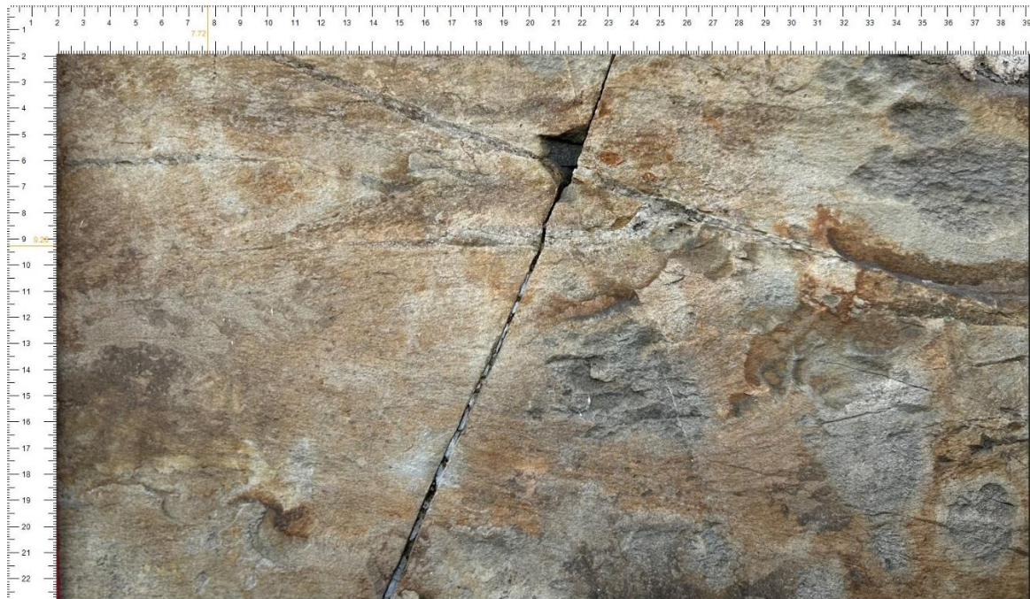
Figure 4.41 Crack image used to determine the extent of damage using image processing.
