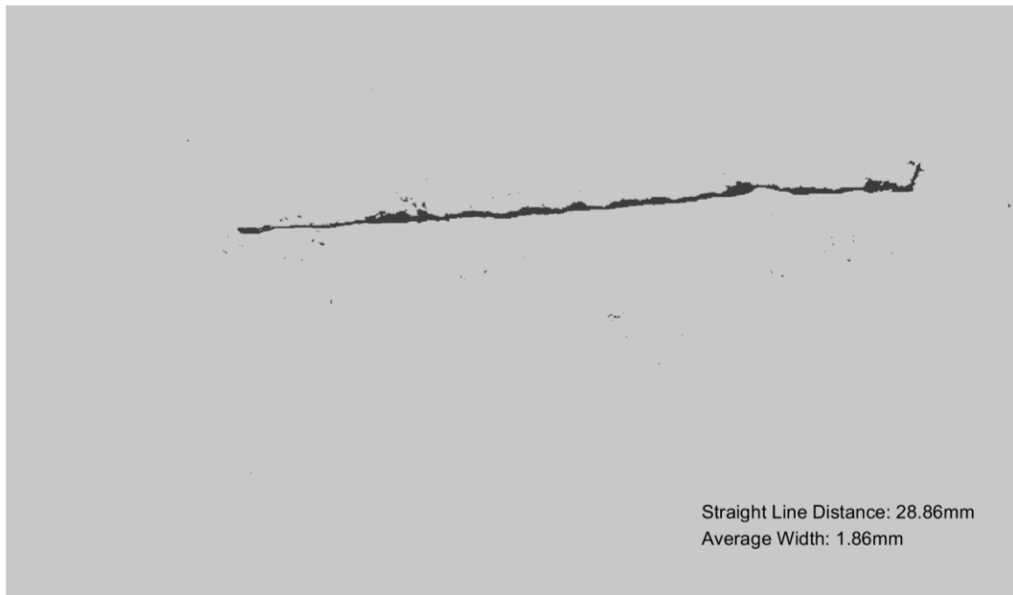
Figure C.7 Linear crack length and average crack width obtained for crack "g".
