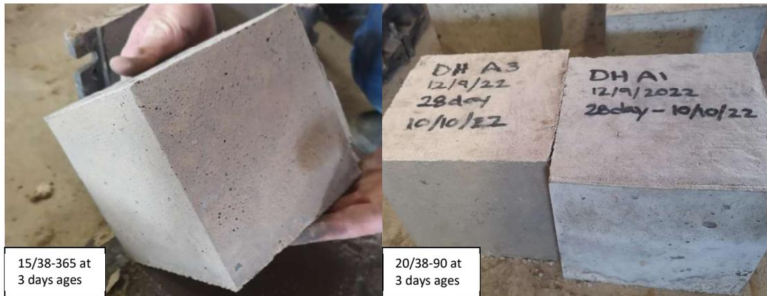
Figure 4.2 Specimens from mixture 15/38-365 and 20/38-90 at day 3 of age
