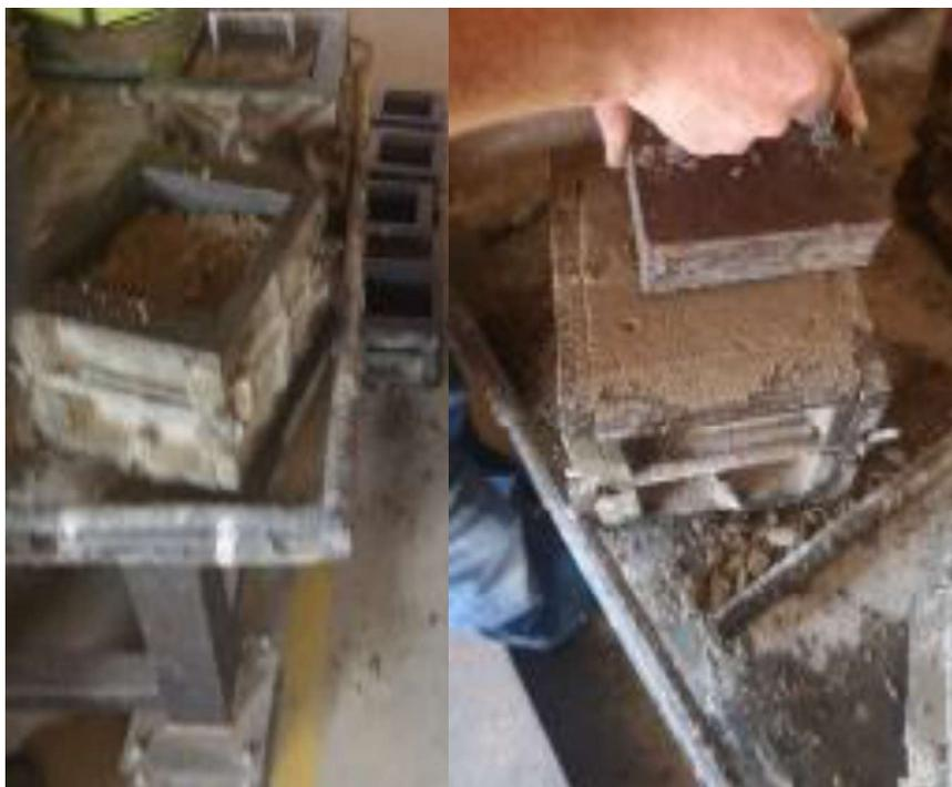
Figure 3.10 Compaction of RCC done on vibration table.
