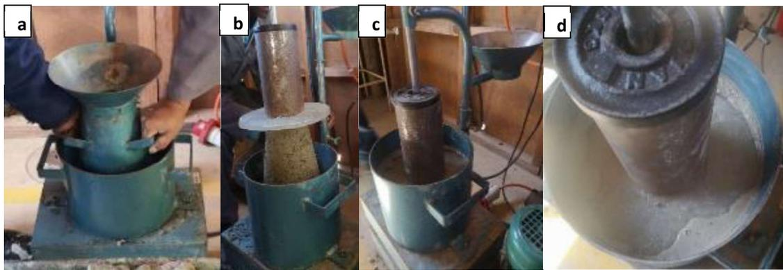
Figure 3.8 Vebe tests done in the laboratory
