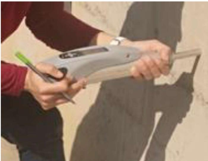
Figure 3.19 Rebound hammer test done on a dam wall in horizontal or 0-degree position
