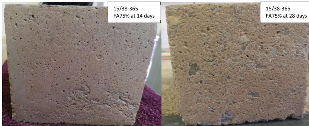
Figure 4.3 Specimens for mixture 15/38-365 FA75% at day 14 and day 28 of age
