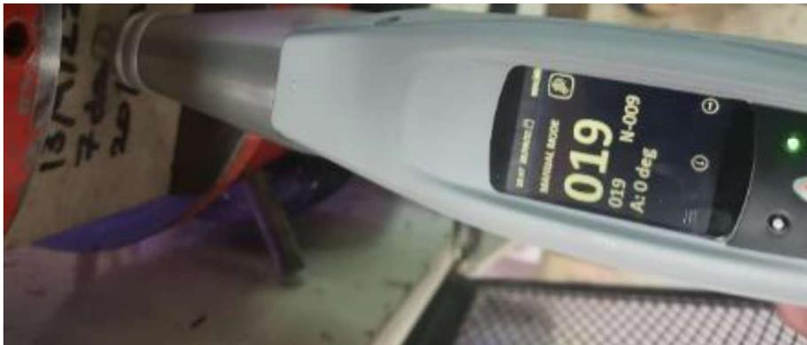
Figure 3.14 Top view from Rebound hammer test done on a specimen in compressive strength machine
