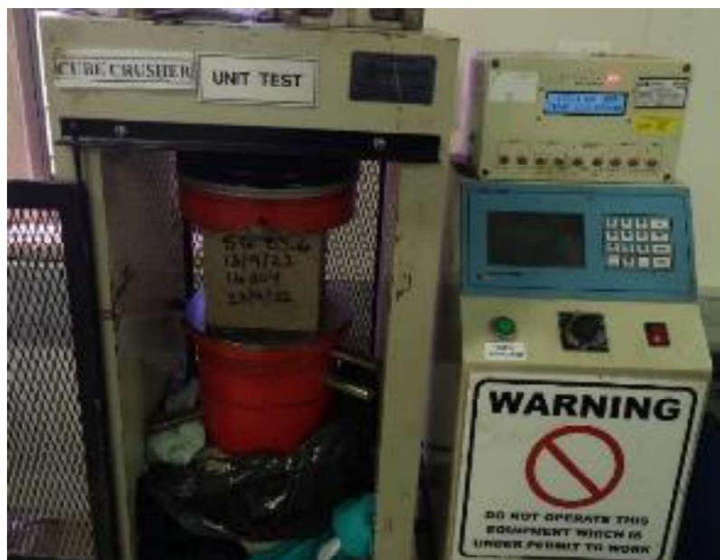
Figure 3.7 Compressive strength test machine
