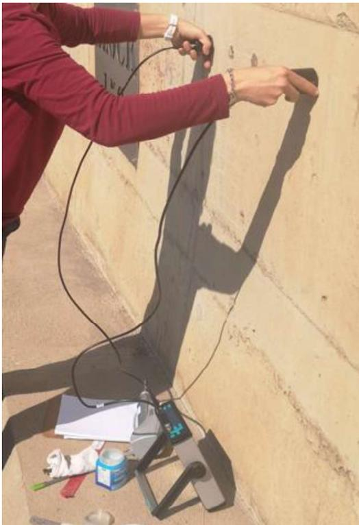
Figure 3.17 Indirect UPV measurement taken at De Hoop Dam wall
