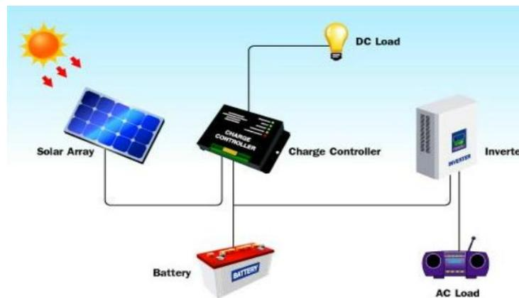
**Figure 3.7:** Elements of the solar energy system (Hassan et al., 2022).
