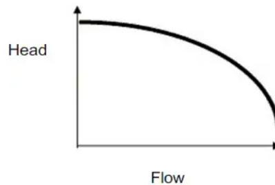
**Figure 3.15: Head and Flow rate Curve (Jalil et al., 2022)**
