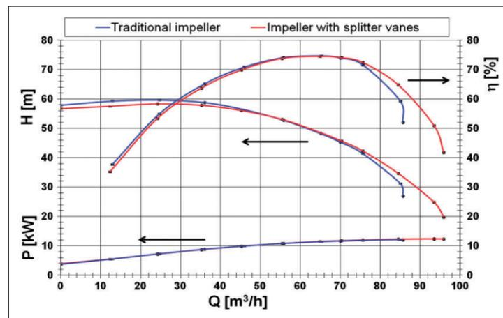
**Figure 3.1:** Performance curves of the centrifugal pumps with and without splitter vanes (Schmitter et al., 2018)
