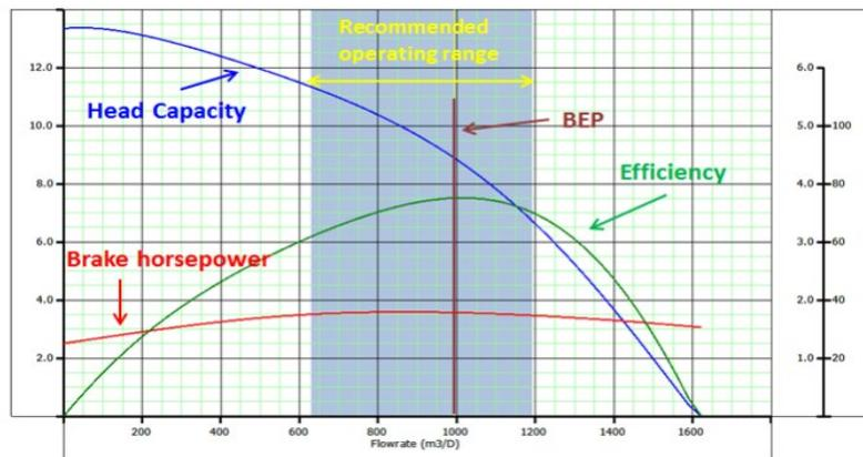
**Figure 3.16:** Typical Pump Performance Curve (Naval and Yusta, 2022a)
