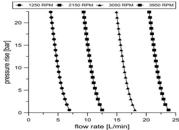
**Figure 3.5:** Operating Curves of the Rotary Vane Pump (Zhou et al., 2020)
