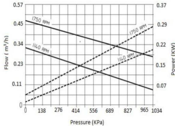
**Figure 3.4:** Gear Pump performance curve (Wei and Sun, 2017)
