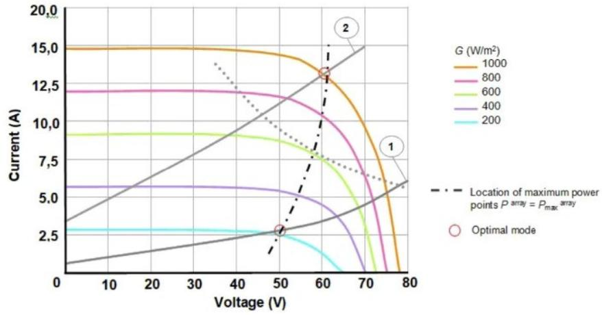
**Figure 2.4:** The family of PV array current-voltage from 0 to 80 V
