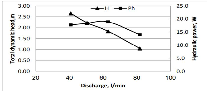
**Figure 3.2:** Performance characteristics curve of Submersible Pump (Fara et al., 2021)
