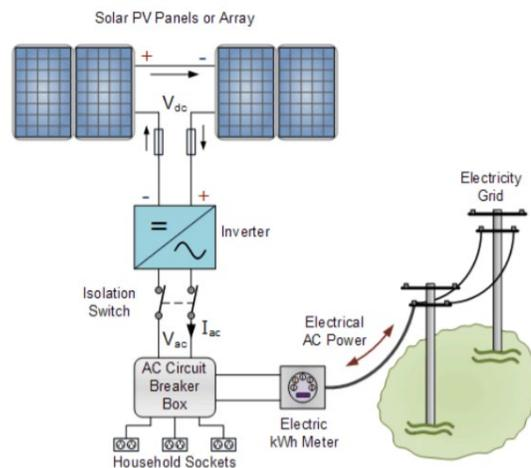
**Figure 3.11: Grid Connected PV System** (Simpson et al., 2021)
