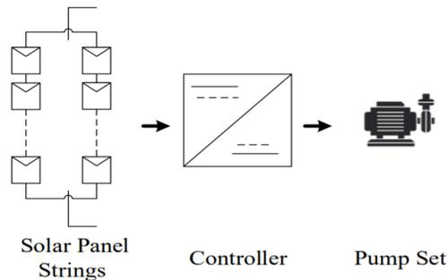
**Figure 3.14:** Block Diagram of the Proposed System (*Bai et al., 2019a*)
