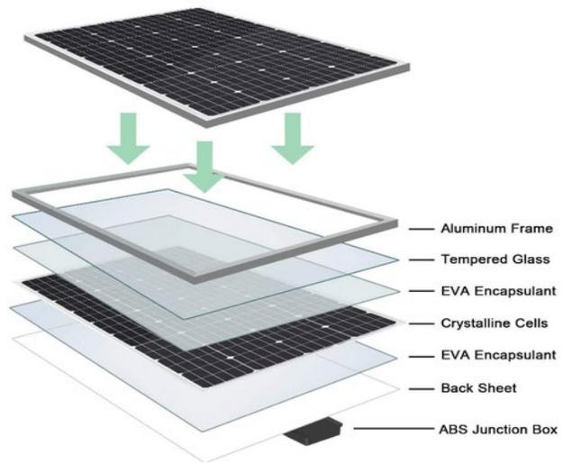
**Figure 3.8:** Main Components of the Solar Panel(Yussif et al., 2020).
