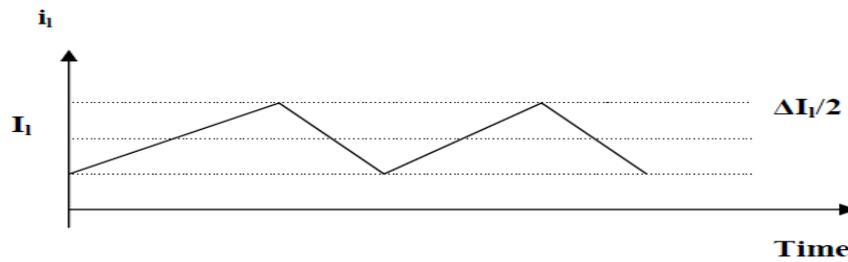
**Figure 4.5: Inductor Currents for Continuous Conduction Mode**
