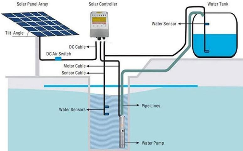
**Figure 4.2:** Configuration of PV Water Pumping System (Jalil et al., 2022)
