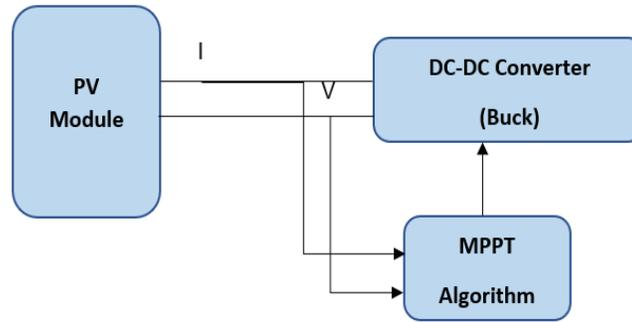
**Figure 4.3:** Block Diagram of the photovoltaic (PV) system
