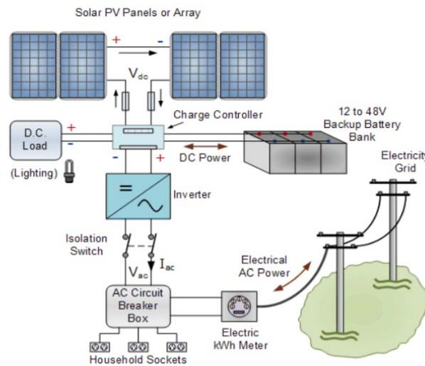
**Figure 3.13:** Grid Tied with Battery Backup (Huang et al., 2020)
