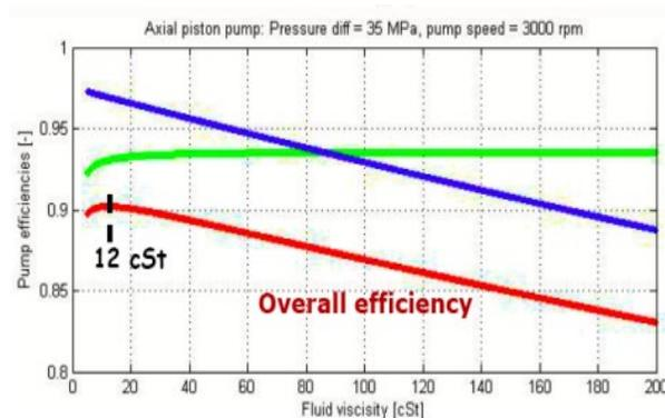
**Figure 3.3:** Efficiencies versus fluid viscosity for Piston Pump at a speed of 3000 rpm (Fara et al., 2021)
