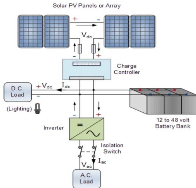
**Figure 3.12: Off-Grid PV System**
