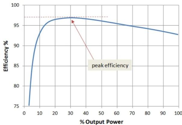
**Figure 3.9:** Inverter's Efficiency Curve (Mitali et al., 2022)
