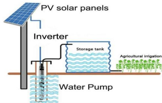
**Figure 3.10: Photovoltaic water pumping system** (Sinapis et al., 2021)
