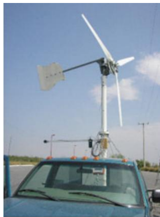
Figure 2.26: Example of vehicle-top test rig (Dawoud et al., 2007)
