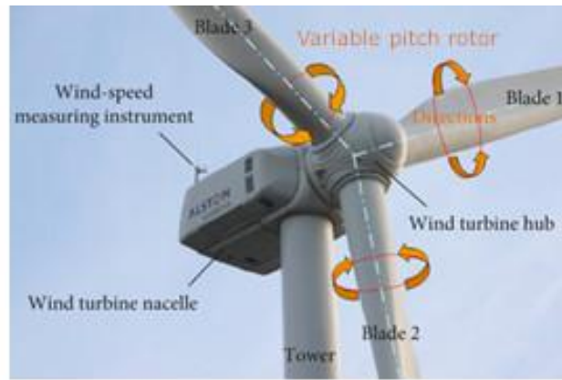
Figure 2.20: Automated pitch control (Adapted from Zhou & Liu, 2018)
