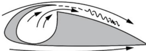
Figure 2.23: Blowing air into the boundary layer (Vos, 2018)
