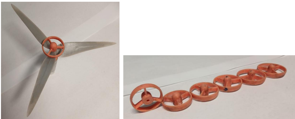
Figure 3.10: 3D resin printed parts: rotor with 15% ring vane (left) and all ring vanes (right)
