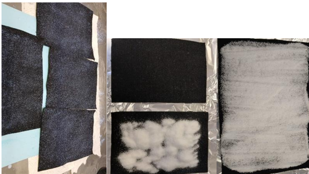
Figure 3.2 (a) Latex and PE powder application
