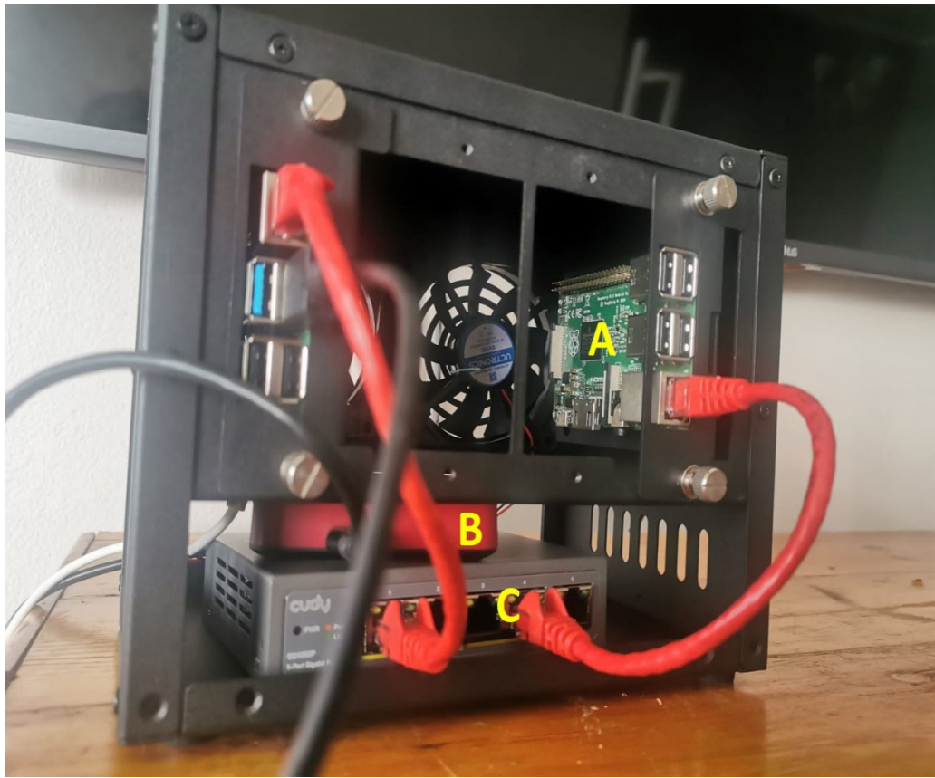
Figure 4.4: Raspberry PI Server Rack
