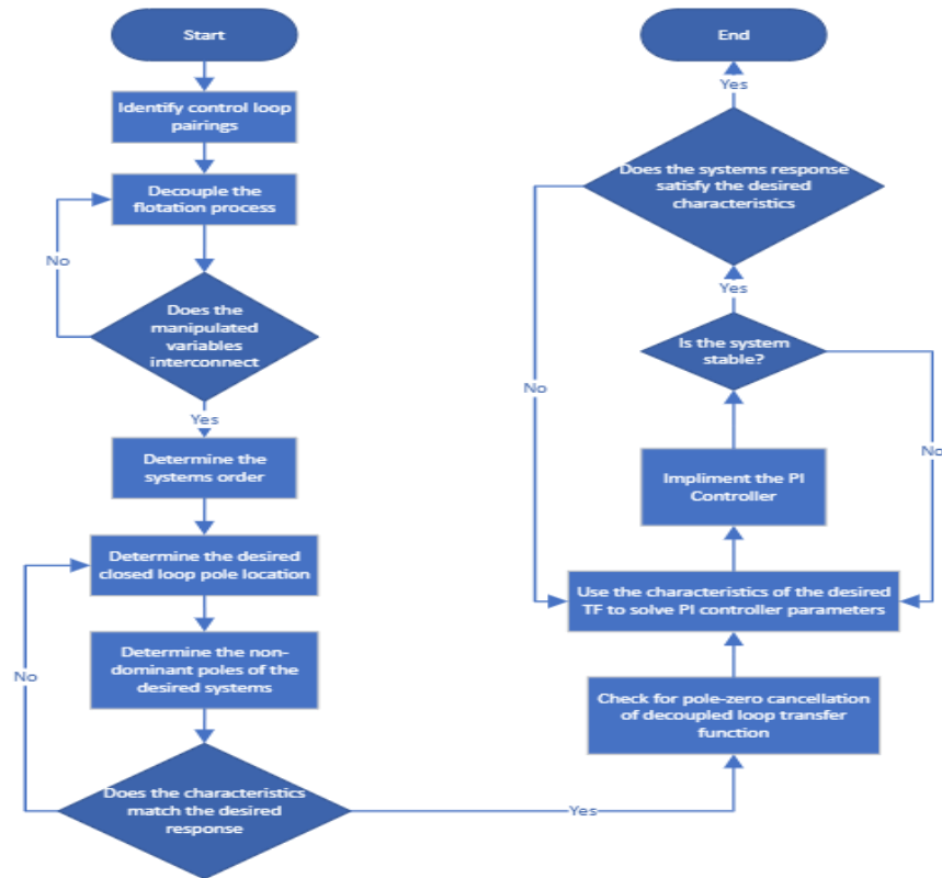
Figure 5.4: Decoupled PI design procedure flow diagram
