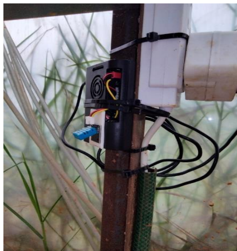
Figure 4.7: DHT22 used to collect ambient temperature and humidity data
