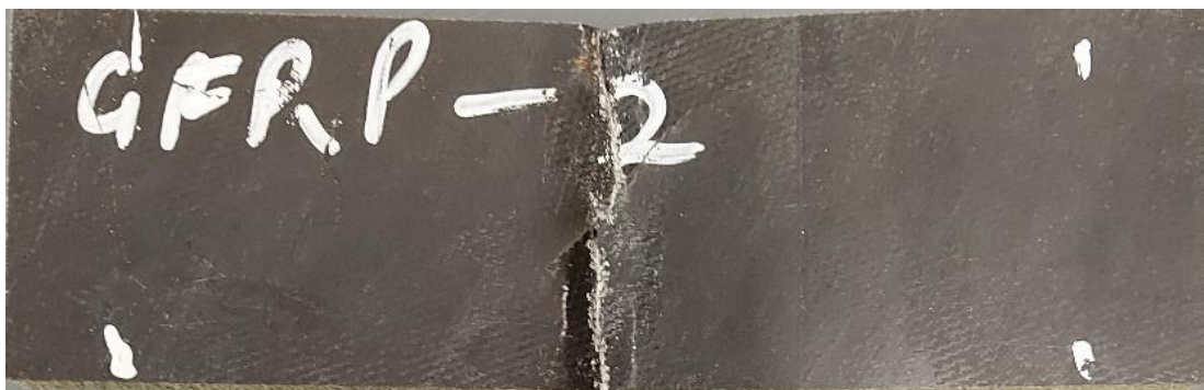
Figure 3.10: Flexure Tested GFRP Specimens
