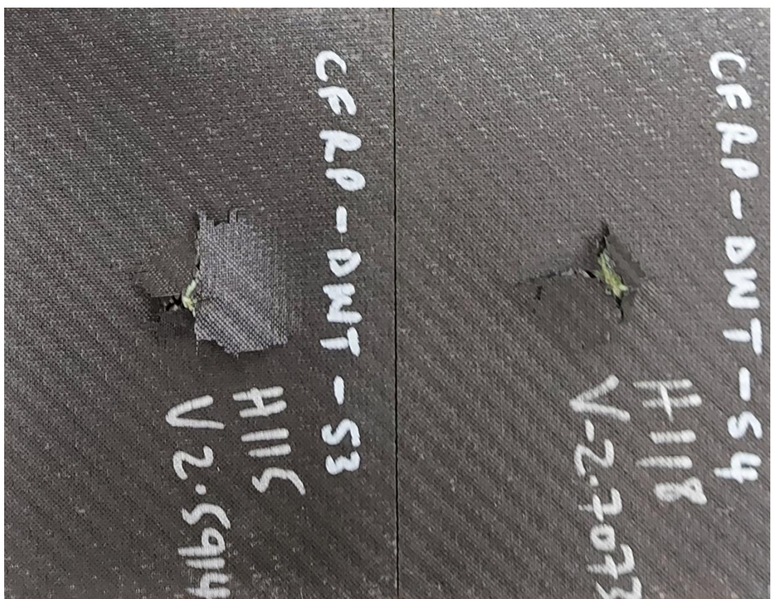
Figure 3.14: Some impacted CFRP specimens
