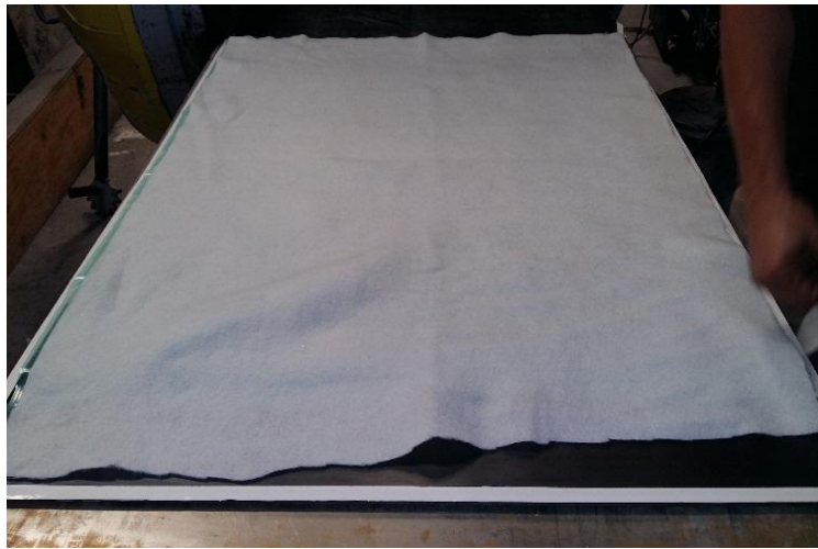
Figure 3.1: Hand lay-up of prepregs
