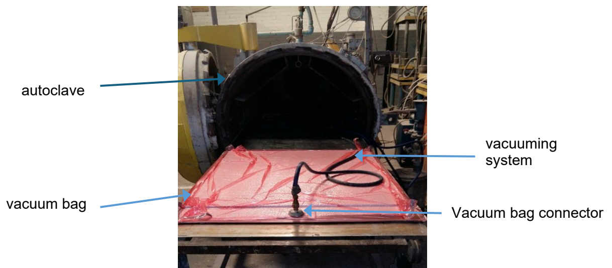
Figure 3.2: Vacuuming process before placing in the autoclave
