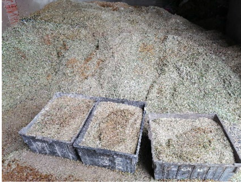
Figure 3.2: 'As-received' waste glass before crushing and sieving
