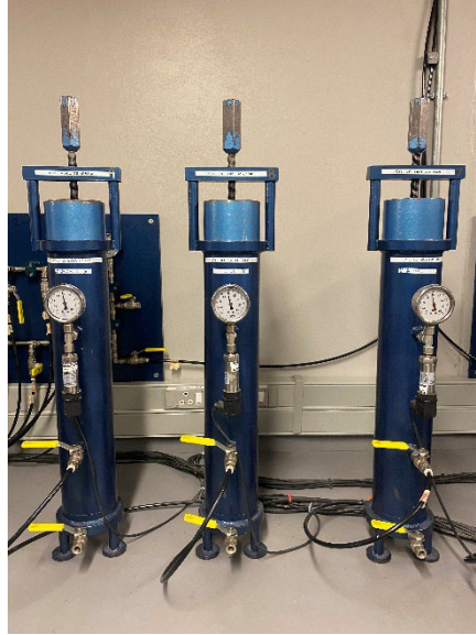
Figure 3.16: Permeameter for OPI tests
