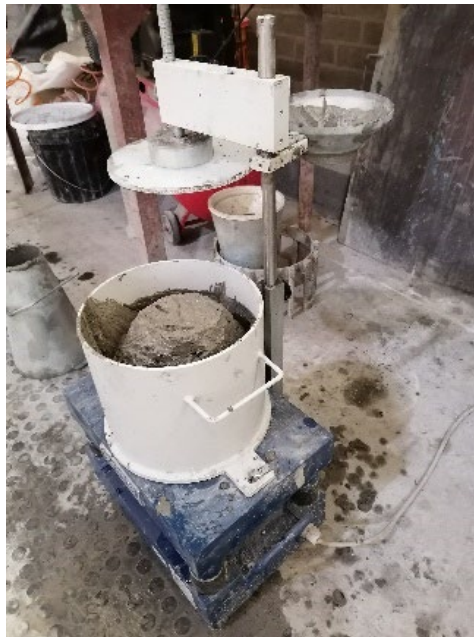
Figure 3.11: Vebe consistometer apparatus
