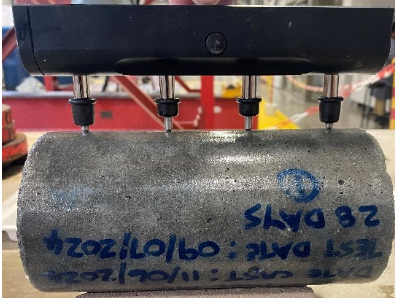
Figure 3.14: Surface resistivity test set-up
