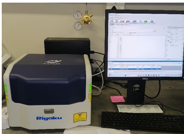
Figure 3.19: Rigaku NEX DE High-Resolution Energy Dispersive X-ray Fluorescence (EDXRF) Spectrometer (UWC laboratory)
