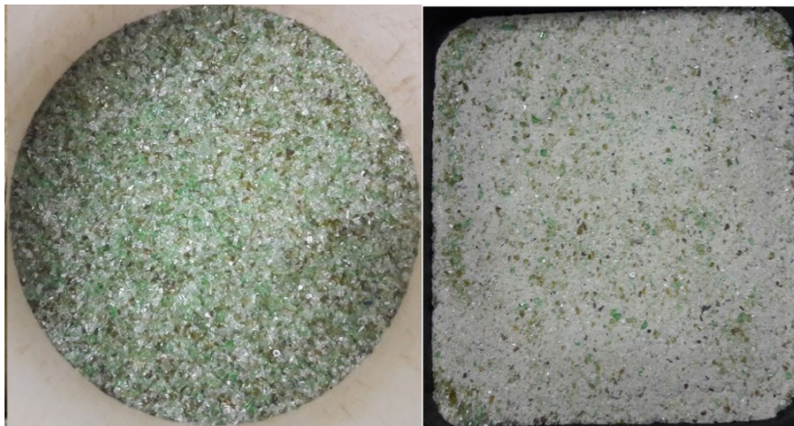
Figure 3.3: Crushing of waste glass to fine aggregate sizes
