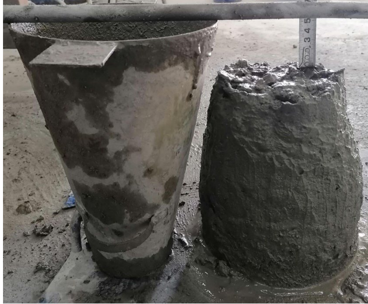
Figure 3.9: Slump test apparatus
