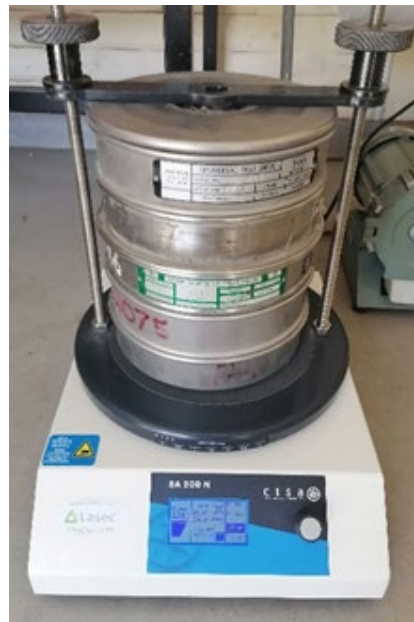
Figure 3.4: Sieve analysis test set-up
