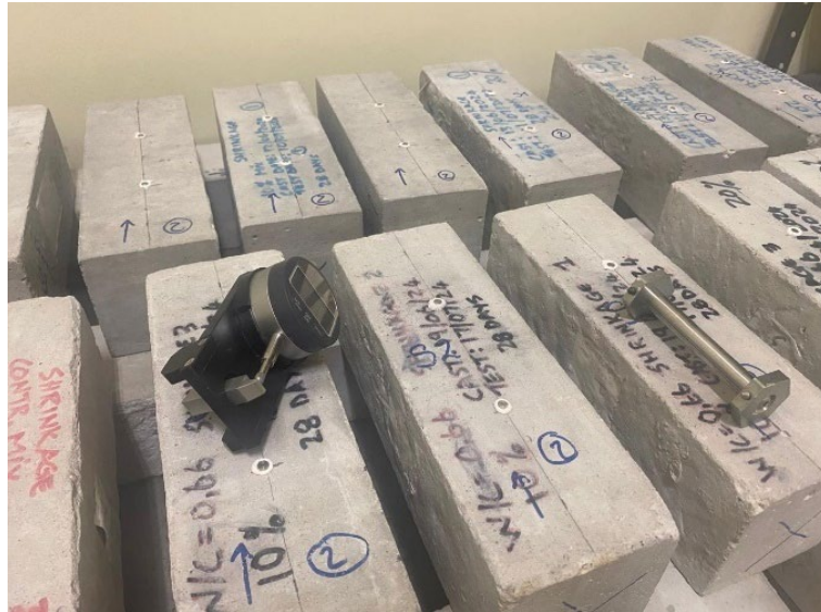
Figure 3.13: Drying shrinkage test set-up
