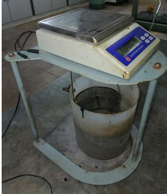
Figure 3.7: Water absorption test set-up
