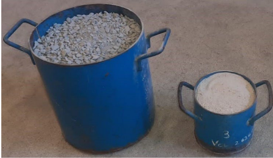
Figure 3.6: Bulk density test set-up
