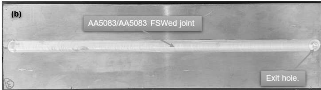
Figure 3.3.1.1.2:(a) FSW performance; (b) AA5083/AA5083 FSWed joint.
