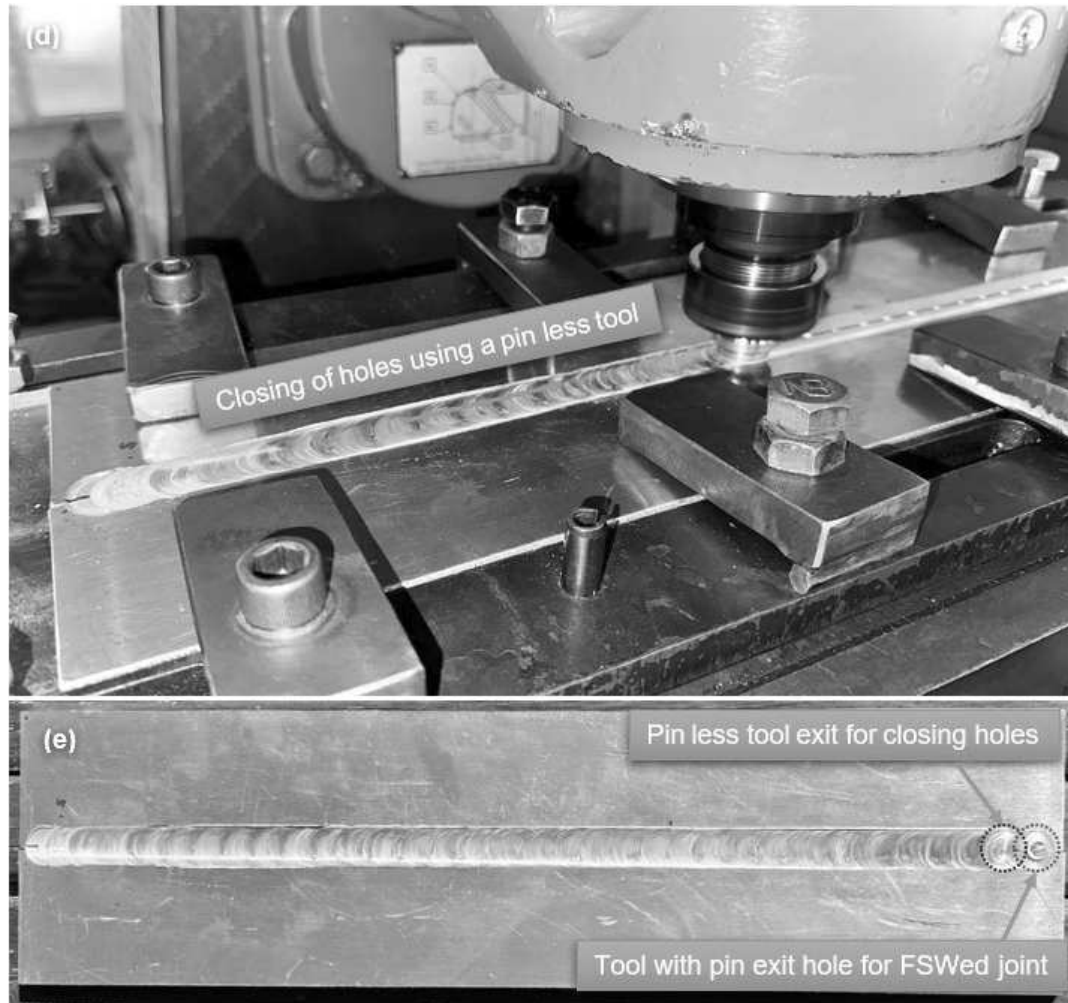
Figure 3.3.1.2: (a) Prepared plate before drilling; (b); Plate after drilling (c); Sample of holes filled with reinforcement particles; (d) Closing of holes using pinless tool; (e) Sample plate after the hole closing process.
