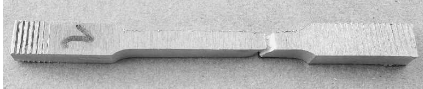
Figure 4.1.5.1: AA5083-H111 base material: post-tensile specimens.
