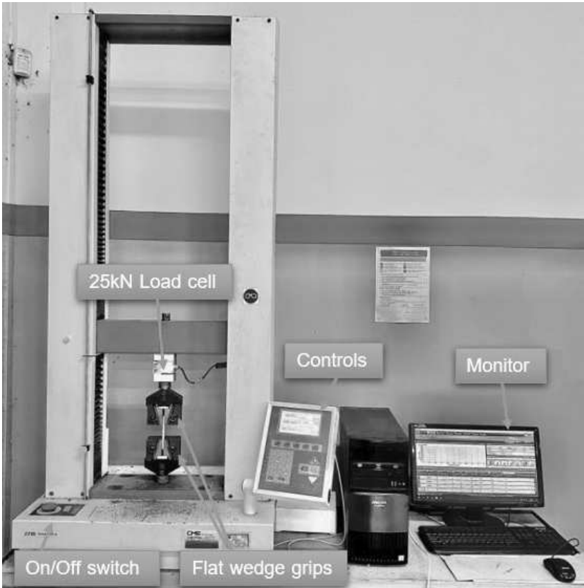
Figure 3.9.1.1: Hounsfield tensile test machine.
