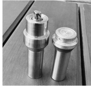
Figure 2. Pin less tool and Pin with tool utilised during the fabrication process.
