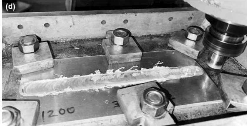
Figure 3.2.2.5.4:(a) Closing of holes using a pinless tool; (b) Sample plate after the hole closing process; (c) FSP Performance for fabricating the composite using a tool with a pin; (d) Sample of AMMCs composite joint.
