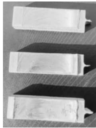
Figure 3.6.1.1: Sample of cut cross-sectional surface joints for microstructure or microhardness specimen.
