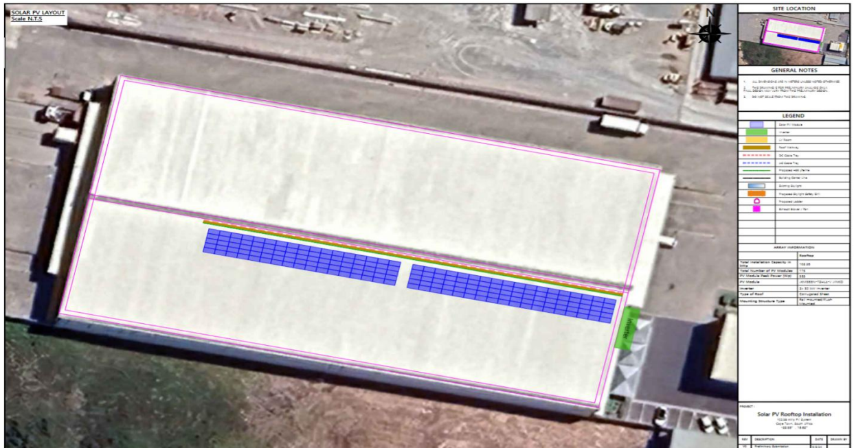
Figure 4.3 Solar PV roof layout.
