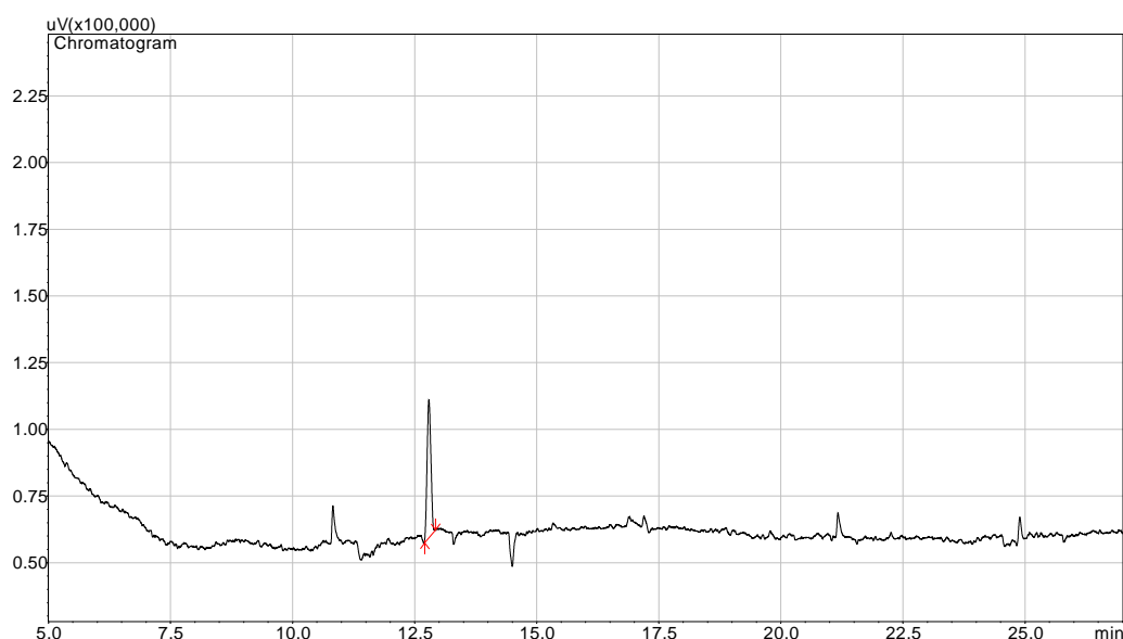
Figure 4.408: Representative TBT chromatogram after adsorption of 100 mg/L TBT with 0.5 g of n\text{Fe}_3\text{O}_4 /fly ash/activated carbon, contact time of 60 min, temperature 20 °C and a stirring speed of 200 rpm
