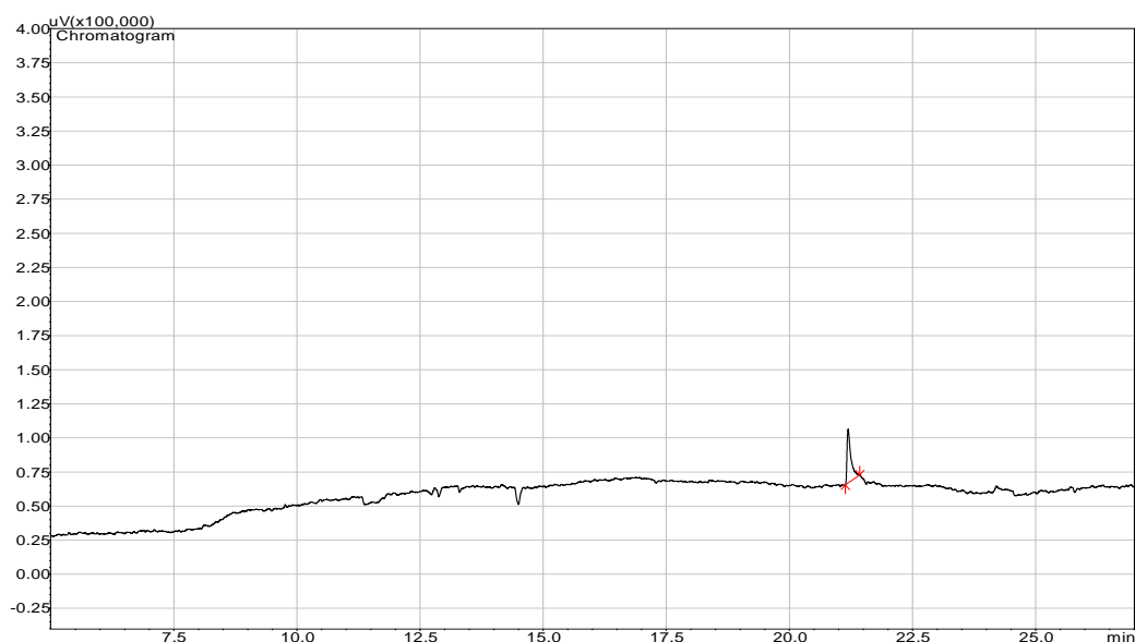
Figure 4.334: Representative TPT chromatogram after adsorption of 100 mg/L TPT with 0.5 g of fly ash/activated carbon, contact time of 60 min, temperature 20 °C and a stirring speed of 200 rpm
